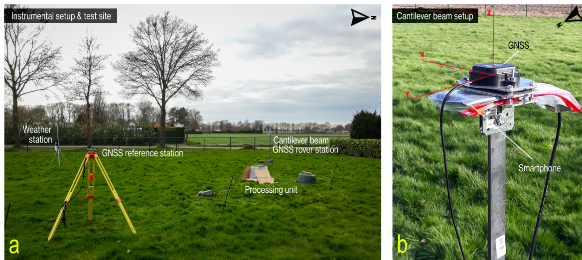
Figure 2. Instrument setup and test site of the ‘Cantilever Beam’ experiment: (a) Overview of the instrument configuration viewed towards west. (b) Rover station sensors alignment at the beam’s top: low-cost GNSS antenna on top with a small metal disc ground plane and smartphone together with plastic cover protection below. The XYZ coordinate system in red coincides with the cardinal East-North-Up (ENU). We will restrict ourselves to the ENU notation in the following.
