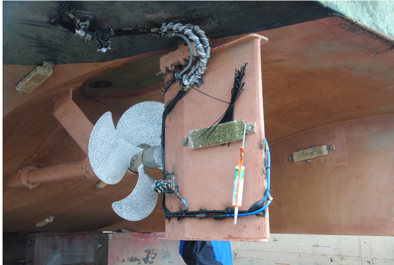
Figure 7: Lights on rudder and hull and cables.
