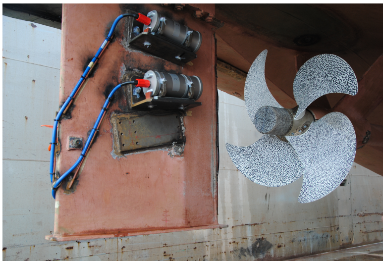
Figure 6: Starboard rudder side with cameras.
