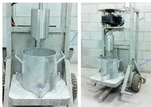
Figure 7. Coaxial cylinder tribometer developed from Feys et al. (2014).
