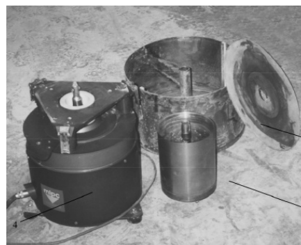
Figure 5. Coaxial cylinder tribometer developed from Kaplan (2001).
