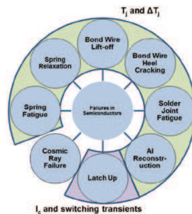
Fig. 5. Failure mechanisms in power semiconductors. From [12].
