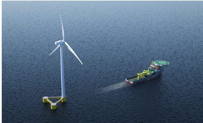
Figure 2-7 Tow of a semi-submersible structure (Energyfacts.eu, 2020)
