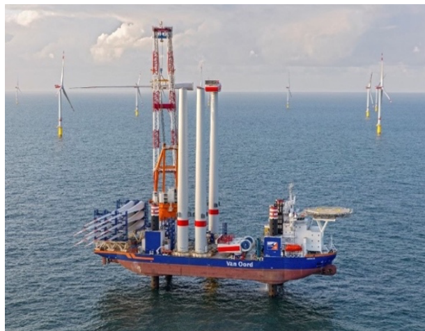
Figure 2-8 Jack-up installation vessel
