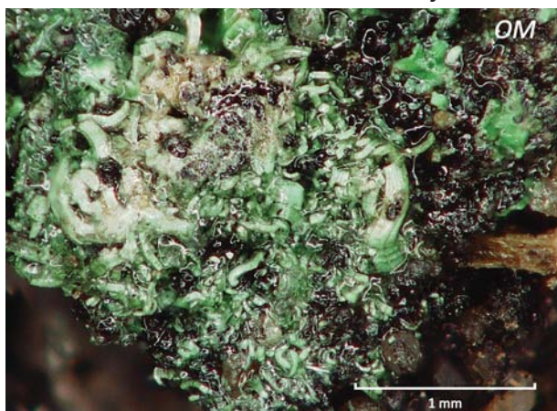
Figure 1: Example of curly malachite as a mass of curls on archaeological bronze from Zevenbergen site. OM: Optical microscope image.
