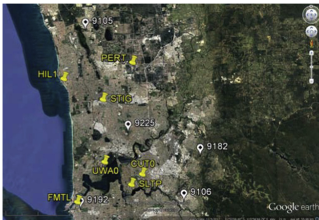
Fig. 1. SF Network A in Perth, Australia with the largest inter-station distance of 30 km. The meteorological stations are marked with white 4-digit numbers. Map data: Google, Data SIO, NOAA, U.S. Navy. NGA. GEBCO, Image © 2018 DigitalGlobe (Google Earth, 2017).
