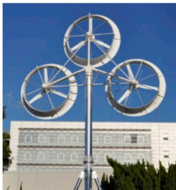
Fig. 9. 10 kW multi-rotor DAWT system installed in Japan. Courtesy of Kyushu University and Riamwind Corporation.
