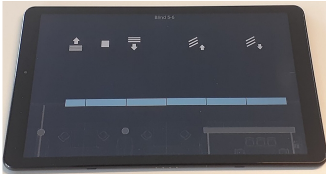
Fig. 6. View of the touchscreen-based controller used by occupants to change the height and the tilt angle of the blinds.
