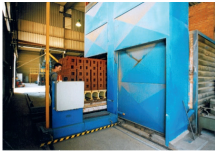
Figure 1: Kiln car with bricks leaving the HZG brick kiln (1997)
