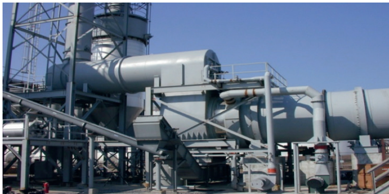
Figure 3. Rotary Kiln close-up. Dewatered sediment with modifiers are charged into the rotating rotary kiln and exit as a melted sediment followed by a water quench to produce a pozzolan beneficial use product called Ecomelt® which is pulverized to make a 30-40% replacement for Portland cement.
