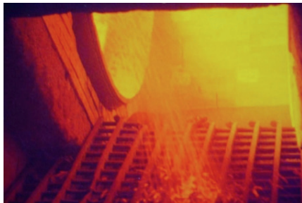
Figure 3: LWA's leaving the Fibo ExClay rotary kiln
