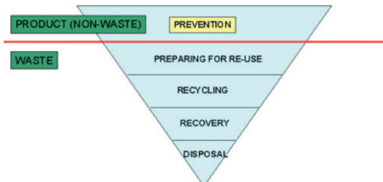
Figure 3 Uncontaminated sediments are a product (non-waste) according to (EU COM, 2008a). Exceeding a contaminant threshold value (one out all out principle) means that sediment is defined as a waste. If sediment treatment is not possible disposal is necessary.
