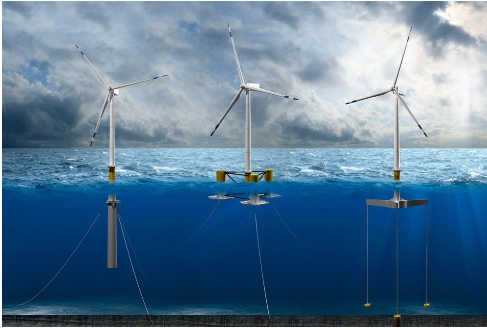
Figure 2.20: 3 different floater concepts from left to right : spar - semi-submersible - TLP. 4
