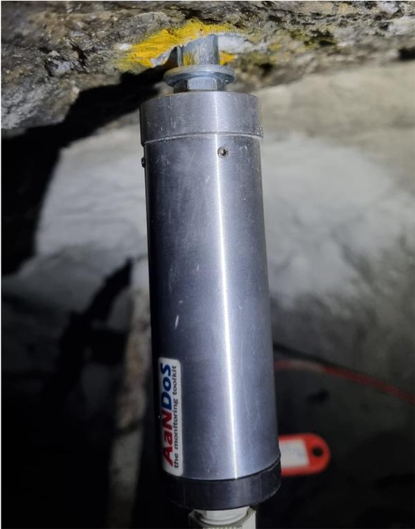
Figure 3.21: AaNDoS geophone connected to a rock bolt.
