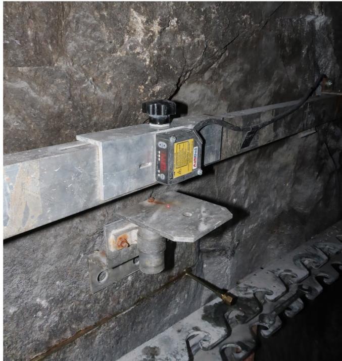
**Figure 3.16:** The laser measuring deformation with respect to the plate attached to the wall.
