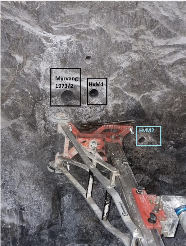
Figure 3.9: The location of the sampling drillholes compared to the old drillhole by Myrvang in 1973.
