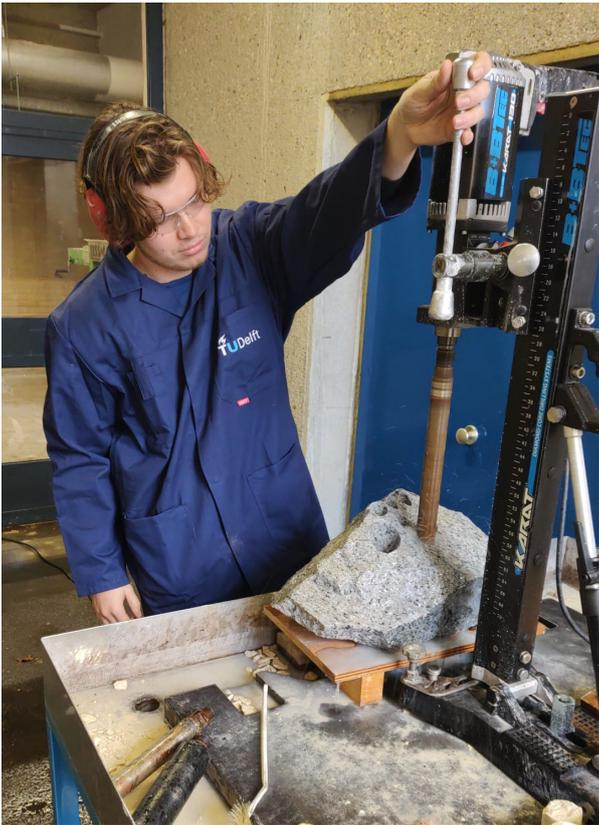
Figure 3.8: The author of this report drilling the samples from a nepheline syenite block.
