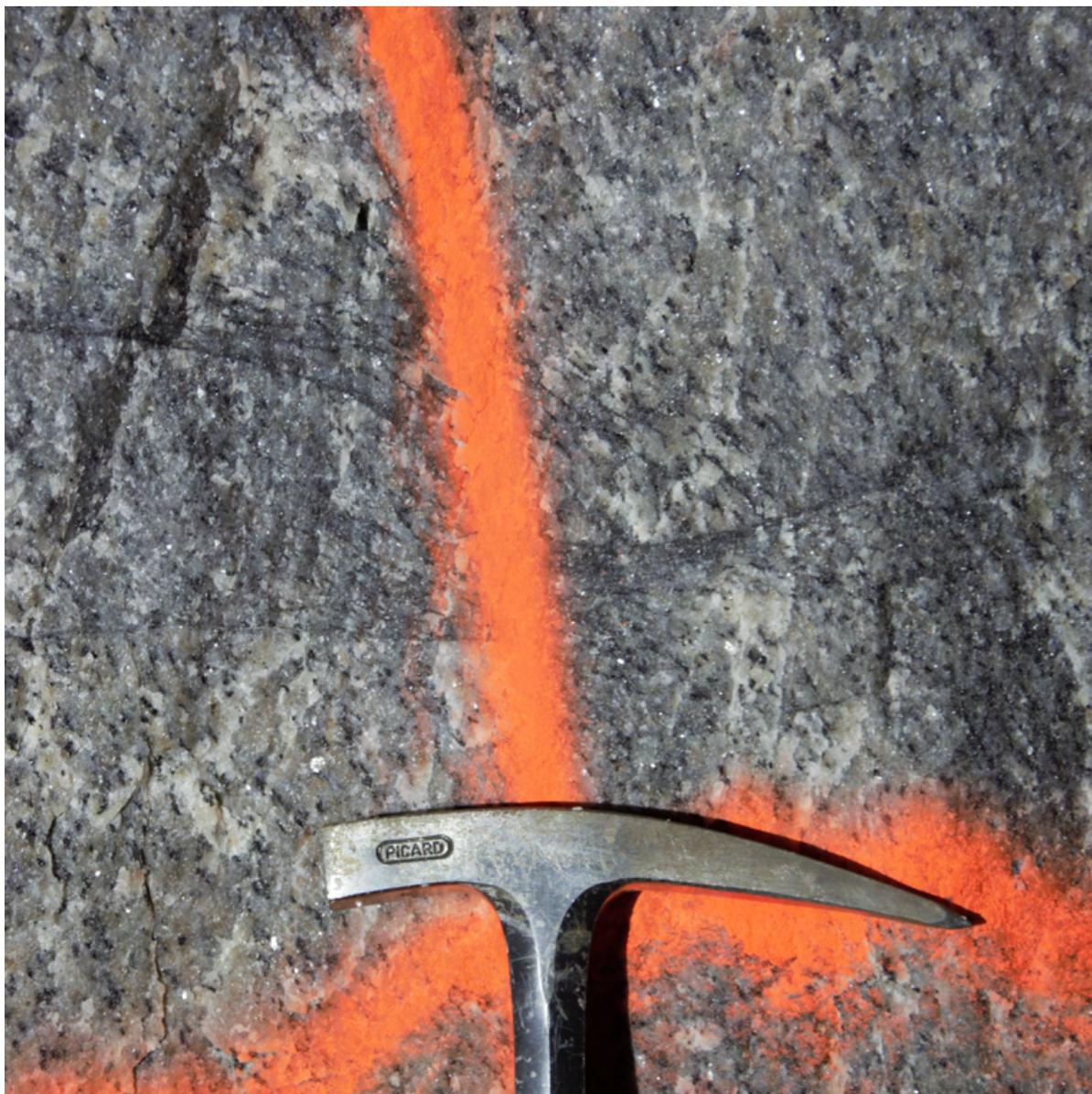
**Figure 2.2:** Lineation of amphiboles in the nepheline syenite at an area subject to spalling (Oostman, 2023).
