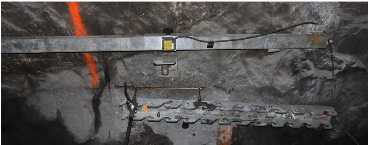
**Figure 3.18:** The set up of the flatjack.
