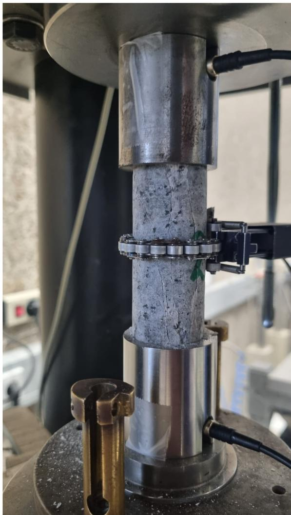
**Figure 3.10:** A (broken) nepheline syenite sample in the set-up as described before.
