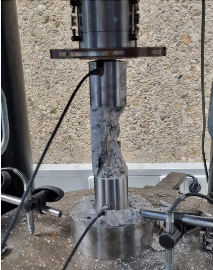
Figure 4.2: The bursting of nepheline-syenite sample HvMCore1 after reaching its UCS.
