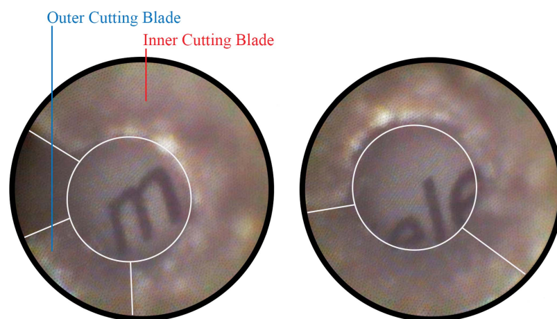
Figure 16. Micro-Endoscopic Images obtained from the Biopsy Needle. In the background a piece of text is illustrated which is imaged using the micro-endoscope.
