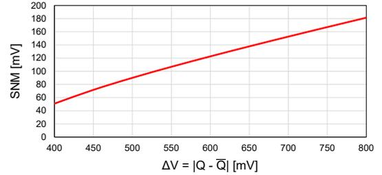
Figure 2. Impact of  $\Delta V$  on the cell's SNM.
