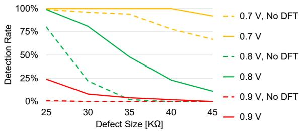
Figure 10. DFT Detection rate for defect BC01.
