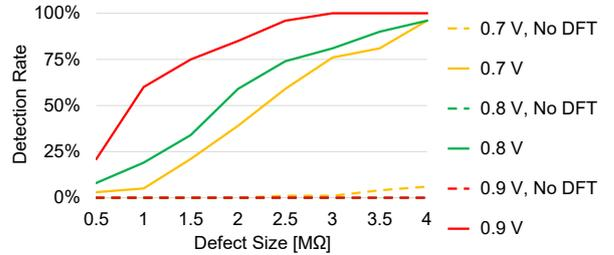
Figure 9. DFT Detection rate for detect OC01.
