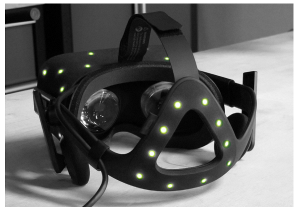
Figure 131 IR LEDs in Oculus Rift headset
