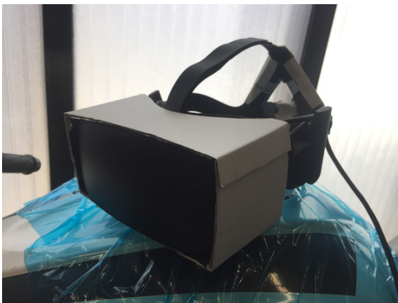
Figure 132 Covering the IR LEDs in the housing and back
