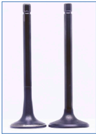
Fig. A13. The initial condition of intake valve and exhaust valve.
