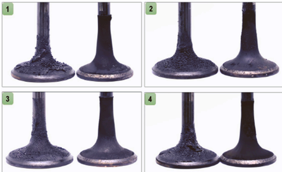
Fig. A14. The condition of intake valve and exhaust valve of the B30 engine after 500 operational hours.
