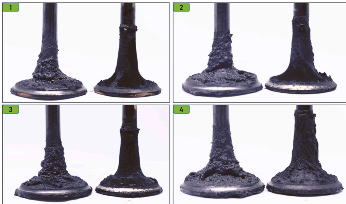
Fig. A17. The condition of intake valve and exhaust valve of the BPO engine after 500 operational hours.
