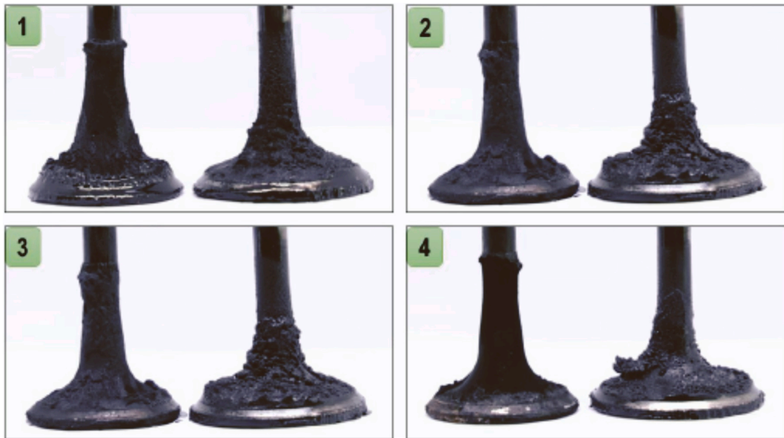
Fig. A15. The condition of intake valve and exhaust valve of the degummed CPO engine after 500 operational hours.
