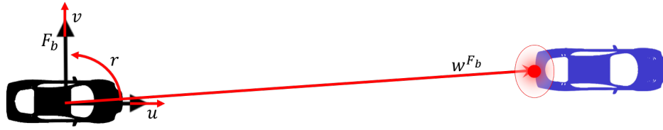
Fig. 2-2: A visualization of the generic vehicle-following field of application. On board of the black follower-vehicle, the Standard Sensor Systems provide the longitudinal velocity u , vehicle yaw rate r and lateral velocity v . In practice, v is not measured but can be estimated or neglected [23]. The local reference frame, attached to the follower-vehicle at time step b , is denoted by F_b . Finally, the Waypoint Source provides the waypoint w^{F_b} used for path generation.
