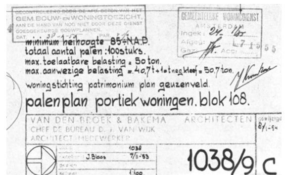
Figure 5.9: Portions of the structural foundation plan for Bouwen Erwoutszstraat. Top image shows a portion of the foundation plan; bottom image the structural pile capacity.
