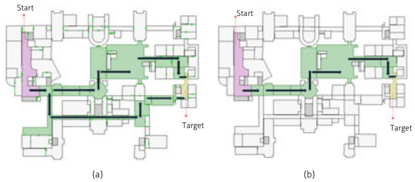
FIGURE 6.15 Routing with two criteria on the logical network of MFA. (a). Two minimum NU paths; and (b) The minimum NU + central HC path.
