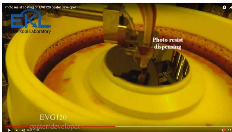
**Figure 4.4** Coating photoresist using EVG 120 <sup>[1]</sup>
