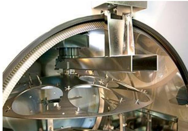
**Figure 4.9** Wafer tray in CHA (face down)
