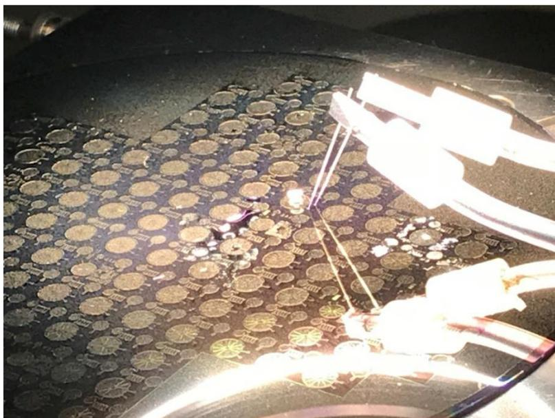
**Figure 5.13** Probe station setup
