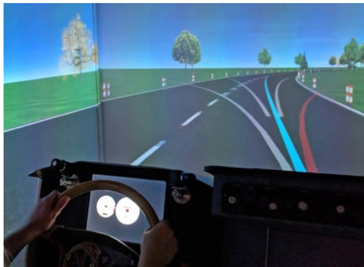
Figure 3.1: Guidance cue in which a trajectory line changes red when it leads outside the road boundaries, adopted from [104].
