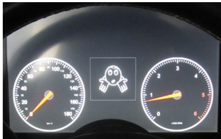
Figure 4.2: Icon shown in the middle to indicate when the ACC is uncertain, adopted from [112].
