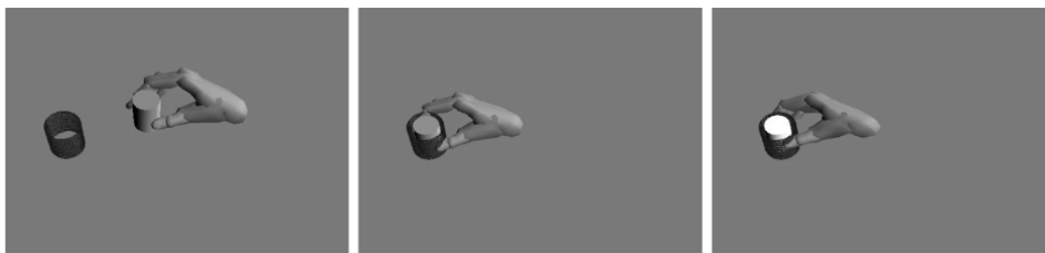
Figure 3.4: Peg in hole task with visual indicator to see when the correct position is reached, adopted from [107].
