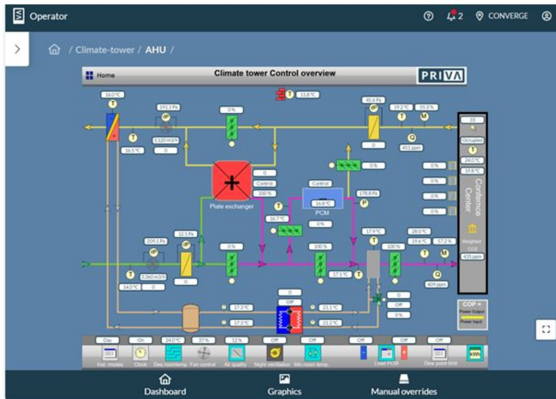
Figure 11: general overview of the BMS-system of the Co Creation Centre. A heat pump, plate exchanger and PCM-battery are visible. Temperatures, CO 2 -levels, relative humidity, air pressure and air flows are measured and presented. Apart from this there is also an energy management module under development.
