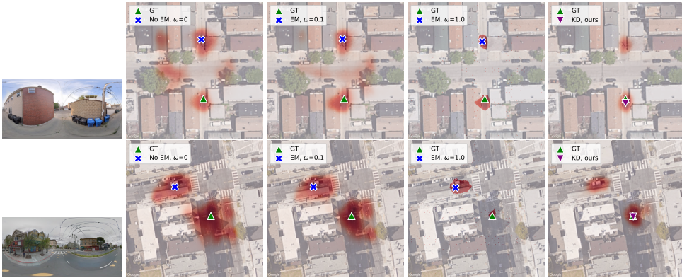
Figure 6.12: Adapting a CCVPE model to the target domain with different methods. Results on the VIGOR test set. Comparison between direct generalization (No EM, \omega = 0 ), different entropy minimization weights (EM, \omega = 0.1 and EM, \omega = 1.0 ), and the proposed knowledge self-distillation (KD, ours). The red color denotes the localization probability (a darker color means a higher probability).
