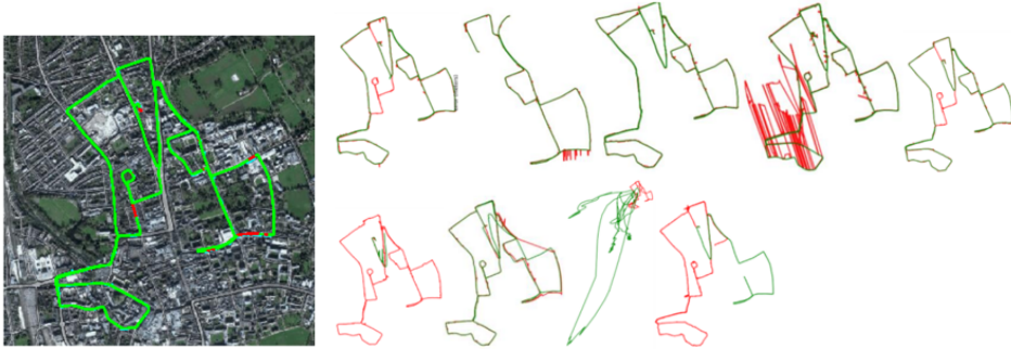
Figure 1.2: Measured trajectories in the Oxford RobotCar dataset [1]. Green: RTK measurements. Red: GNSS measurements. Note that, the selected trajectories are not labeled with “poor GPS” in the original dataset.
