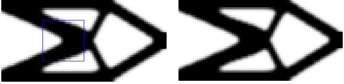
(a) Final design \bar{x}_{\text{ref}} after standard optimization of cantilever beam, with compliance c_{\text{ref}} = 100 and redesign domain in blue.
