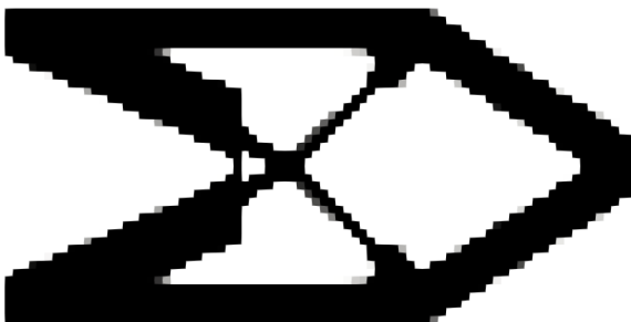
(e) Final design x after local redesign of Fig. 3.4a, with compliance c = 7117.2 and v_{max}=20\% .
