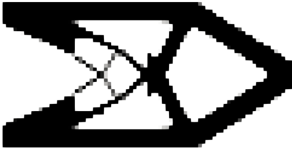
(a) Final design x after local redesign of Fig. 3.4a, with compliance c = 135.8 and v_{max}=20\% .
