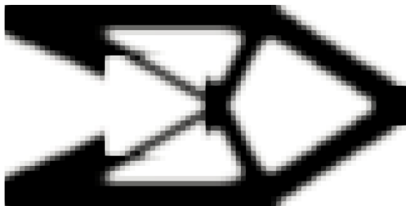
(a) Final design \bar{x} after local redesign of Fig. 3.6a, with compliance c = 184.3 and v_{max}=20\% .
