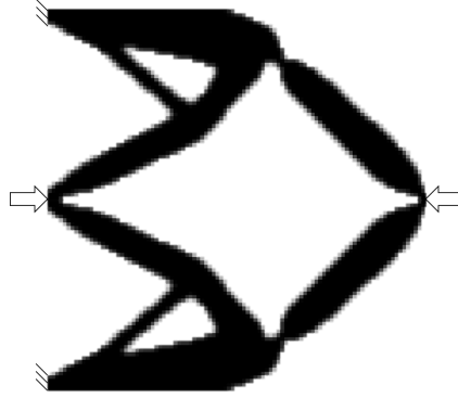
Figure 1.4: Compliant force inverter, generated using the 88-line MATLAB-code of [2]. The direction of the input force (left arrow) is inverted at the output (right arrow).
