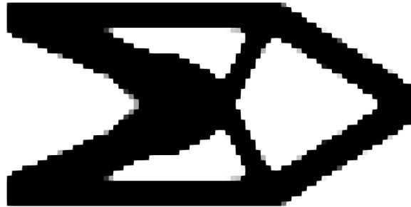
(d) Final design x after local redesign of Fig. 3.4a, with compliance c = 90.13 and v_{max}=86\% .
