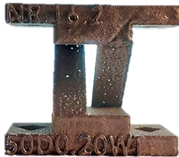
Figure 2.12: Pores in the flexures of a CAFP with FT = 200 \mu\text{m} and OA = 50°.
