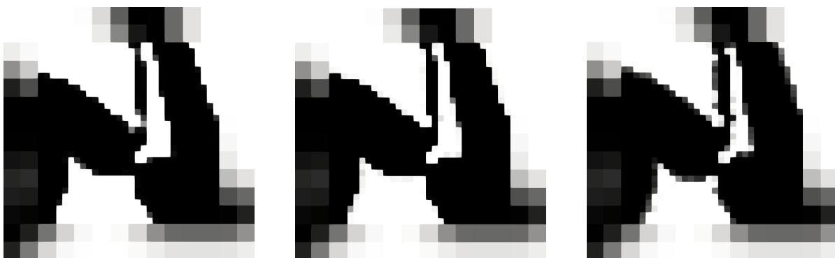
(a) Close-up of eroded projected densities of redesign region, with robust formulation.
