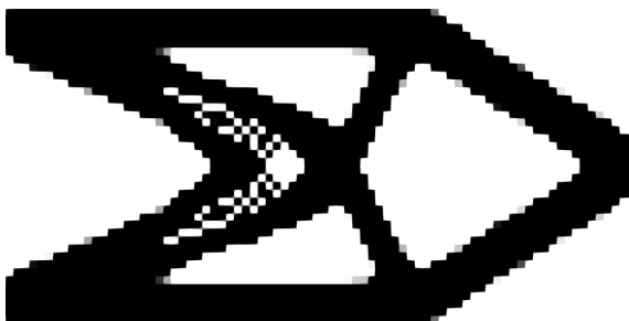
(c) Final design x after local redesign of Fig. 3.4a, with compliance c = 93.78 and v_{max}=66\% .
