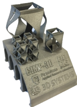
(a) Inconel 625 cellular contact-aided compliant mechanisms designed for stress relieve, reprinted from [44].
