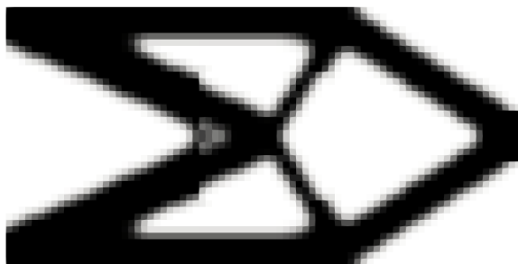
(f) Final design \bar{x} after local redesign of Fig. 3.6a, with compliance c = 106.2 and v_{max}=50\% .
