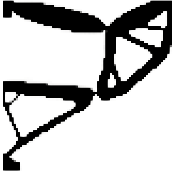
Figure B.13: Intermediate projected densities of robust optimization after 300 iterations of CM design case.
