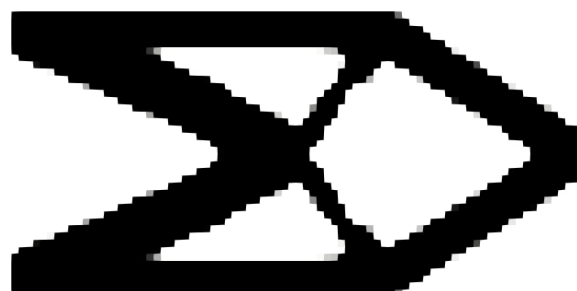
(f) Final design x after local redesign of Fig. 3.4a, with compliance c = 96.40 and v_{max}=50\% .
