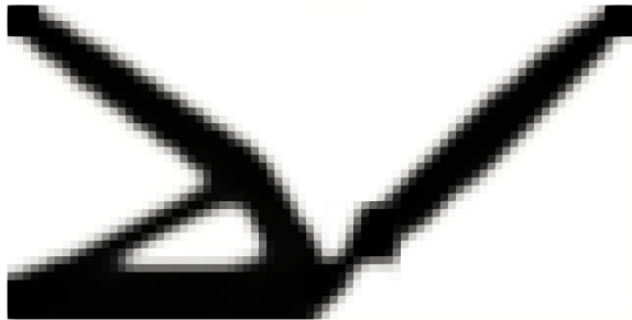
(b) Final design \bar{x}_{ref} after optimization of a compliant force inverter, with u_{out} = 1.002 and v_{max}=64\% .
