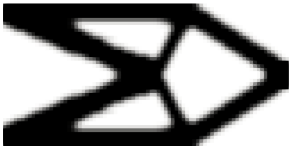
(c) Final design \bar{x} after local redesign of Fig. 3.6a, with compliance c = 102.9 and v_{max}=66\% .
