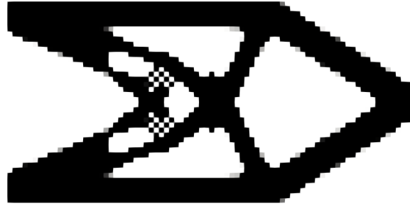
(b) Final design x after local redesign of Fig. 3.4a, with compliance c = 100.1 and v_{max}=50\% .
