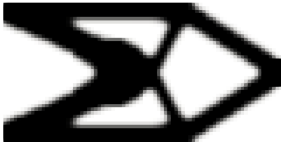
(d) Final design \bar{x} after local redesign of Fig. 3.6a, with compliance c = 98.16 and v_{max}=86\% .
