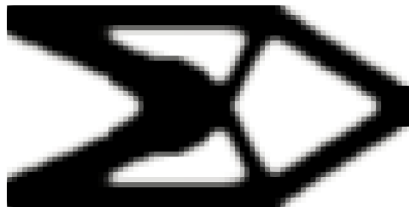
(d) Final design \bar{x} after local redesign with static condensation of Fig. B.8a, with compliance c = 98.13 and v_{max}=86\% .
