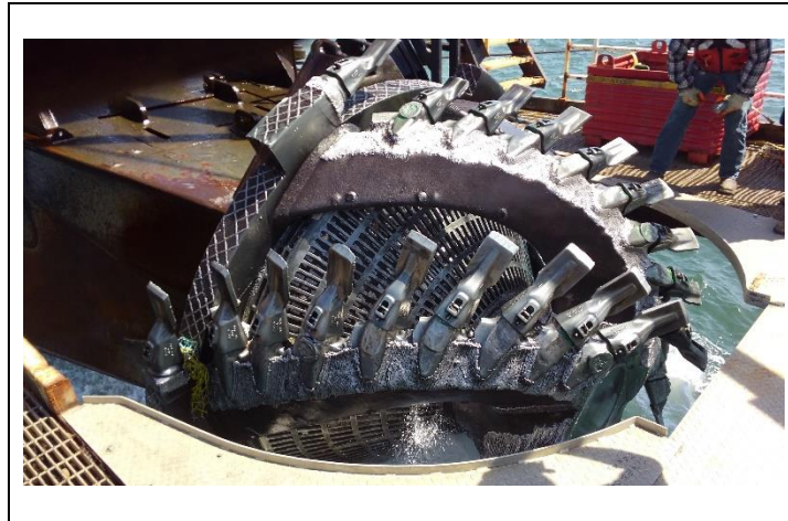
Figure 2: Cutter head (screened) of The Texas (GLDD)
