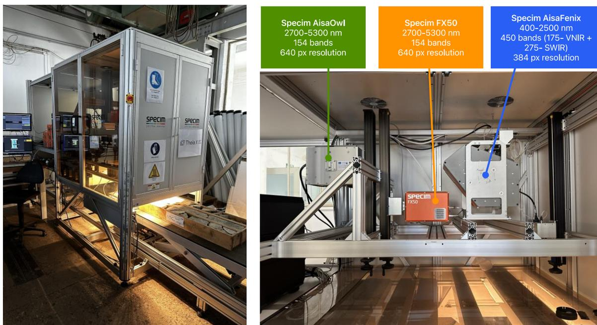
Figure 4.2: SisuROCK drill core scanner (left) with mounted sensors (right) in the visible to near-infrared and shortwave infrared (VNIR-SWIR), mid-wave infrared (MWIR), and long-wave infrared (LWIR) range.
