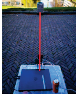
(b) Experimental setup for radome design, the radar has a front aluminum plate.
