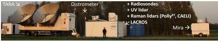
Figure 3.1: Measurement setup of the ACCEPT campaign at CESAR. The arrows point on the TARA radar (radar on the left), the disdrometer that is mounted on the LACROS container, and the vertical pointing Mira cloud radar (35 GHz). Complementary instruments of ACCEPT are listed but not visible on this photo.
