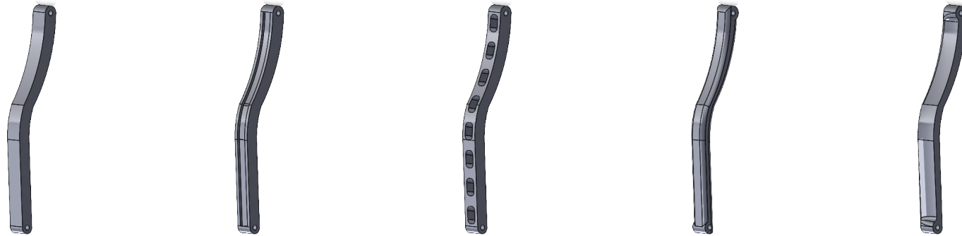
Figure 62: From left to right: 1.Original Rod, 2.Rod with an I-Profile, 3.Rod with Cutouts, 4.Rod with Filleted Edges, 5.Rod with a Neck Shape
