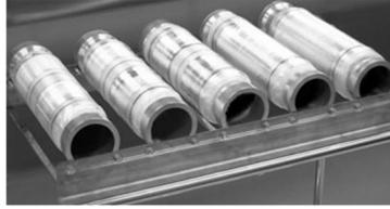
Figure 2.1: Roll of silicone dielectric electro active polymer
