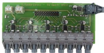
Figure 6.12: Optical fibre link adjustment board
