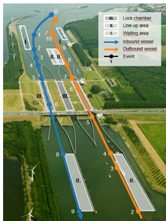
Figure 1 The Volkerak lock complex with highlighted infrastructural elements that are critical for modelling the vessel behaviour (logistics) during lock passages. Critical elements and events are numbered (image by F.P. Bakker & M. van Koningsveld, is licenced under CC BY-SA 4.0, the background image was retrieved from https://beeldbank.rws.nl , Rijkswaterstaat).
