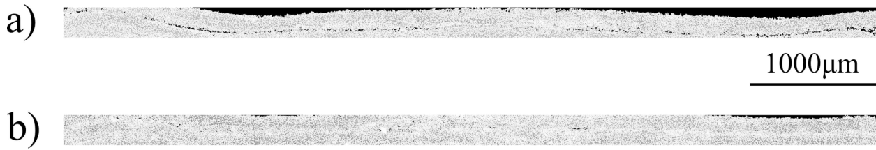
Fig. 12. Examples of cross-sectional micrographs of the topmost interface. a) low intimate contact (80.3%, at 1750 W and 100 N) b) high intimate contact (95.6%, at 1750 W and 1000 N).
