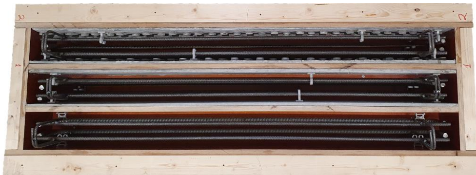
Figure 33 Mould for two hybrid beams and reference beam (the first series of the beams)
