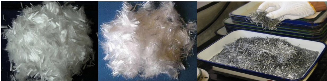
Figure 7 Photo on the left: Polyvinyl Alcohol (PVA) fibres [21]. Photo on the centre: High Modulus Polyethylene (HMPE) fibres [22]. Photo on the right: steel fibres [23].
