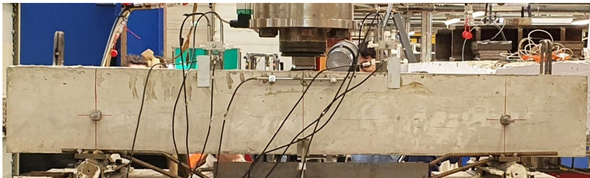
Figure 49 Side views of the beam with smooth laminates with the configuration of LVDTs.
