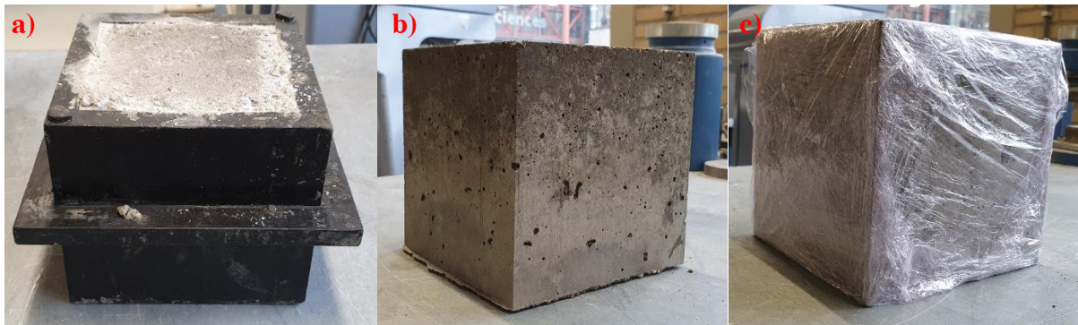
Figure 43 Normal concrete cube specimen 150 \text{ mm} \times 150 \text{ mm} \times 150 \text{ mm} . a) cube in mould; b) perspective view of concrete cube; c) sealed cube specimen.
