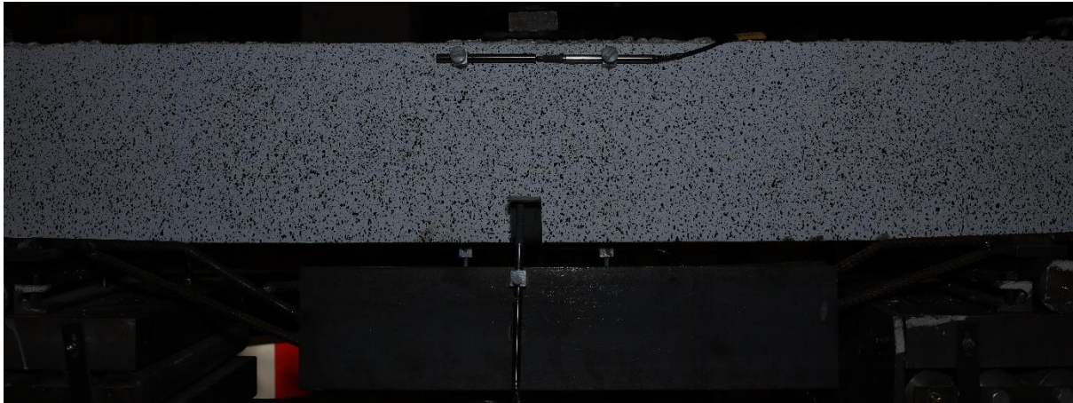
Figure 55 The speckle pattern with LVDTs on the reference beam with shear reinforcement for DIC.
