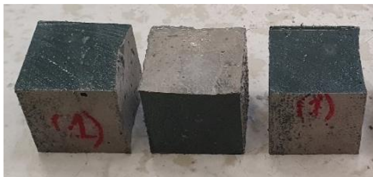
Figure 39 SHCC cube specimens 40 mm × 40 mm × 40 mm
