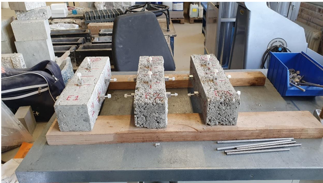
Figure B-1 Three normal concrete prism specimens with a dimension of 400 × 100 × 100 mm 3 [the second series].
