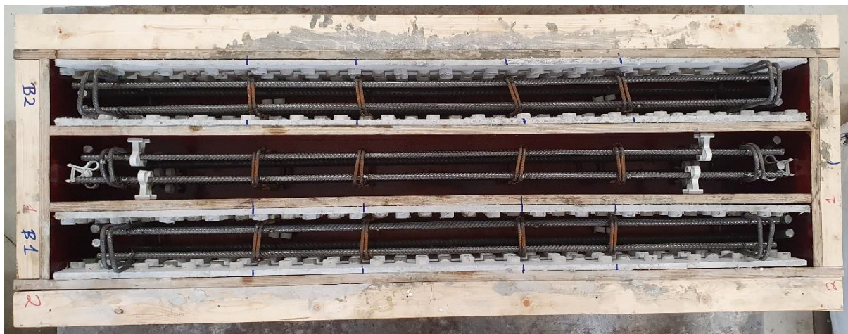
Figure 37 Mould for two hybrid beams and reference beam (the second series of the beams)
