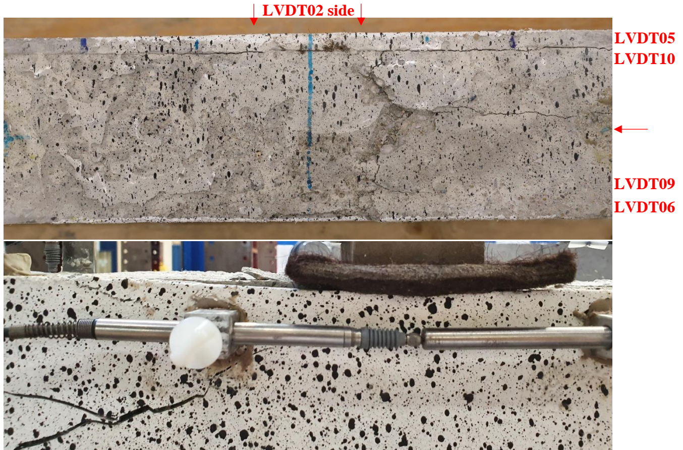
Figure 92 The close-up on final cracks of the hybrid beam B2 with shear reinforcement. Top picture: the top view of the load application. Bottom picture: the side view near load application.
