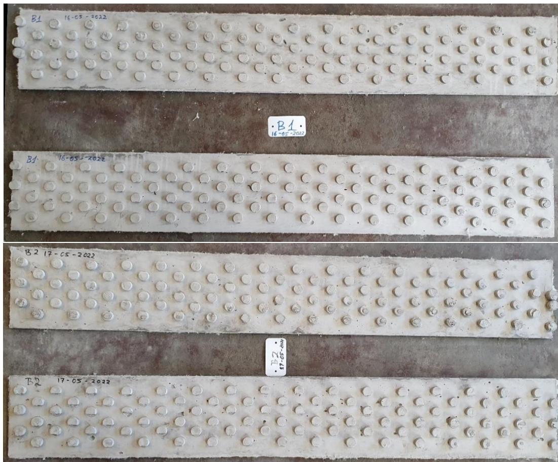
Figure 36 SHCC laminates with shear keys (the second series of the beams)
