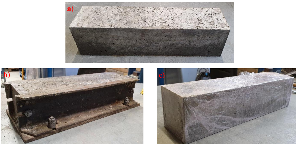
Figure 44 Normal concrete prism specimen 400 \text{ mm} \times 100 \text{ mm} \times 100 \text{ mm} . a) perspective view of concrete prism; b) prism in mould; c) sealed prism specimen.
