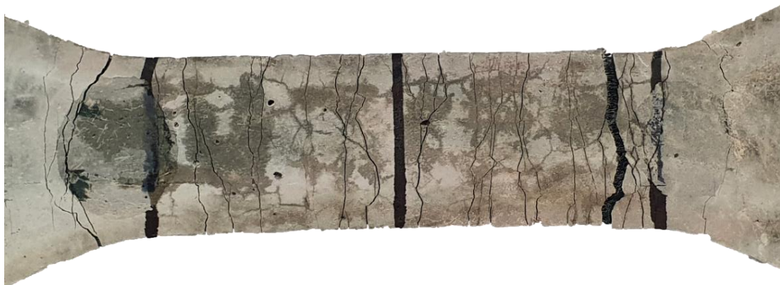
Figure 66 The crack pattern of SHCC. Specimen: B1_d1_56.
