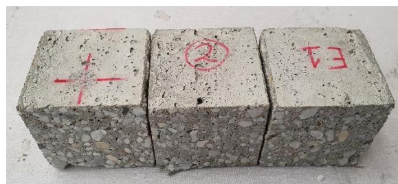
Figure 45 Normal concrete cube specimens 100 \text{ mm} \times 100 \text{ mm} \times 100 \text{ mm}
