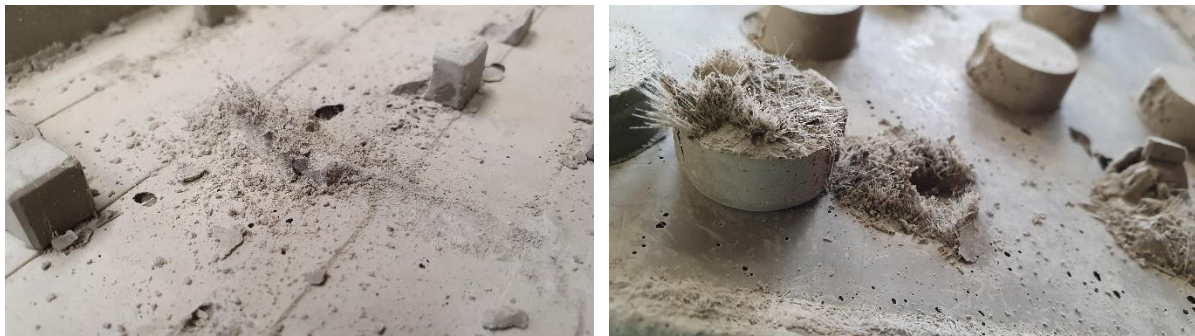
Figure B-1 Close up of profiled laminate. On the left: removed shear key with dimensions 10 mm × 80 mm. On the right: removed shear key with diameter of 25 mm.
