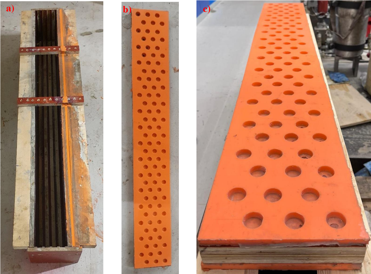
Figure 29 a) Mould for rubber mesh. b) Single rubber mesh. c) Rubber meshes glued on formwork board.
