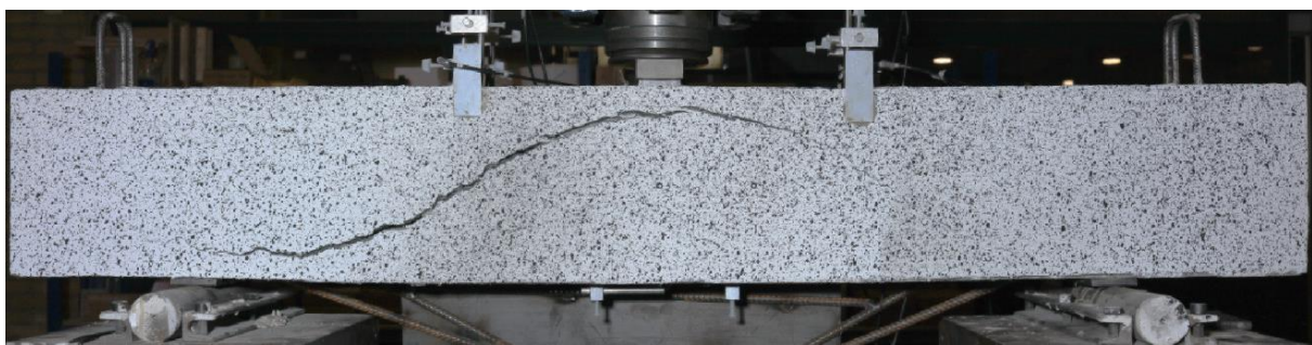
Figure 75 Final crack pattern of the beam with smooth laminates {back side}
