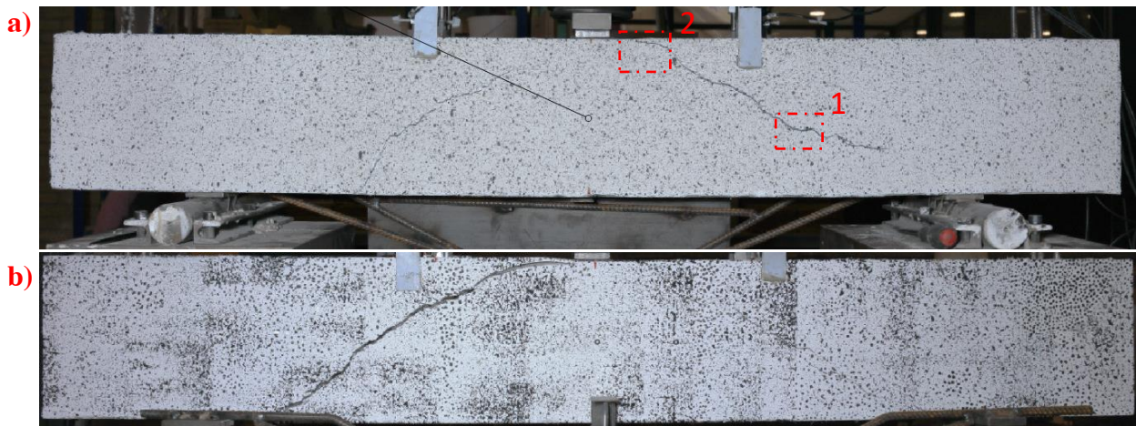
Figure 77 Final crack pattern of beam with shear keys laminates (a) K1 and (b) K2 side view.
