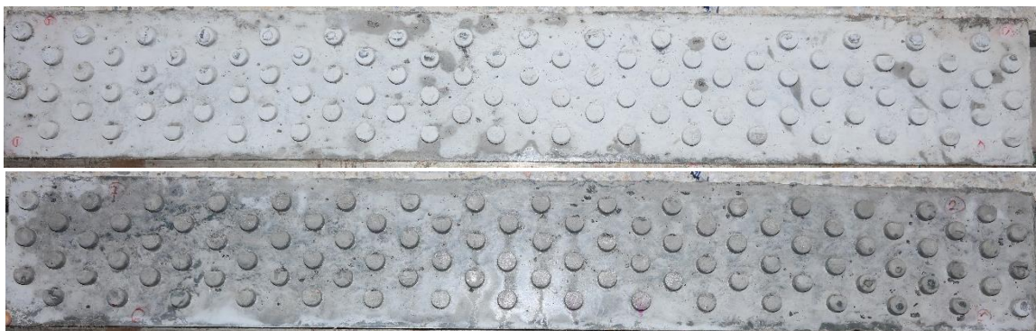
Figure 31 SHCC laminates with shear keys (the first series of the beams)
