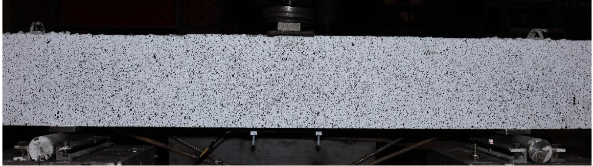
Figure 54 The speckle pattern on the reference beam with shear reinforcement for DIC.
