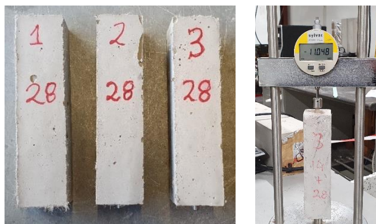
Figure 42 Left: SHCC prism specimens (150 mm × 40 mm × 40 mm) for shrinkage test. Right: Setup for length measurement of a prism specimen.
