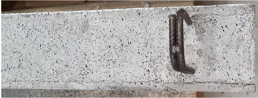
Figure 88 Partial delamination of laminates prior to testing. The bottom laminate (in this picture) is the laminate which delaminated completely during the test.
