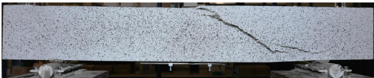
Figure 73 Final crack pattern of reference beam without transverse reinforcement
