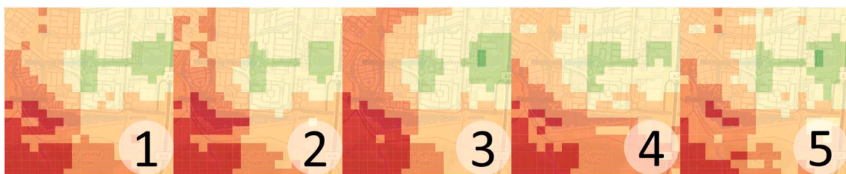
Fig. 5. The output of the method application for a selected part of the region, shown for scenario 1 to 5. Green cells have a high hub potential, red cells have a low hub potential.
