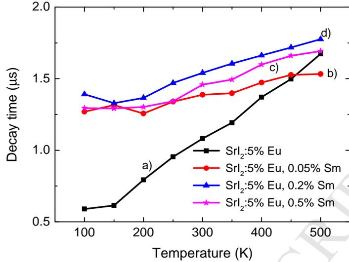
FIG. 6: Temperature dependence of the scintillation decay time constant of  $\text{SrI}_2:5\% \text{Eu}^{2+}$  with a) 0%, b) 0.05%, c) 0.2% and d) 0.5%  $\text{Sm}^{2+}$ . The scintillation decay time constants are obtained by fitting the decay profiles with a single exponential component.
