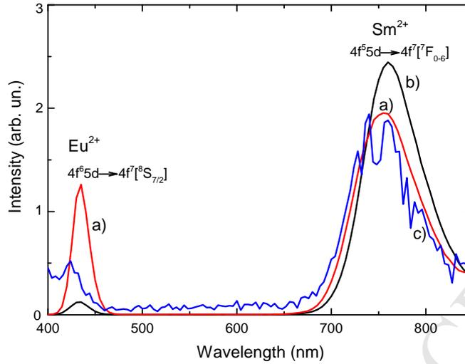
FIG. 2: Normalized X-ray excited luminescence spectra of SrI<sub>2</sub>:5% Eu<sup>2+</sup> with a) 0.05%, b) 0.2% and c) 0.5% Sm<sup>2+</sup> measured at room temperature.
