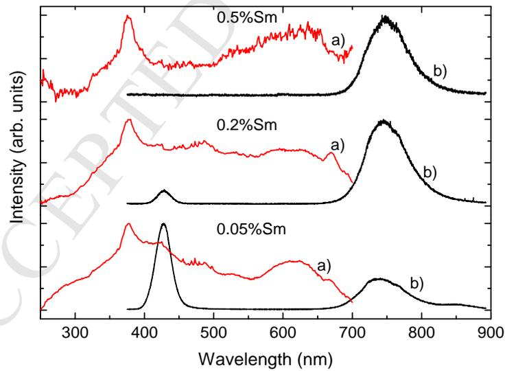
FIG. 4: Photoluminescence excitation spectra a) of 740 nm emission, and b) emission spectra at 370 nm excitation of  $\text{SrI}_2:5\% \text{Eu}^{2+}$  with 0.5%, 0.2% and 0.05%  $\text{Sm}^{2+}$  measured at room temperature.
