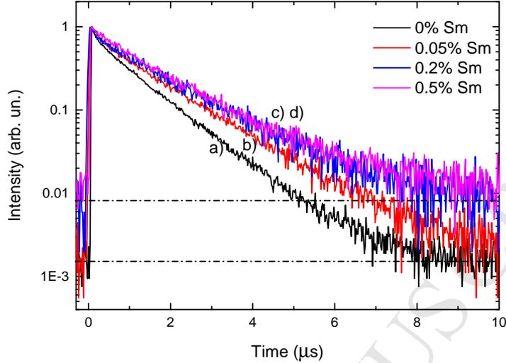
FIG. 5: Scintillation decay profiles of  $\text{SrI}_2:5\% \text{Eu}^{2+}$  with a) 0%, b) 0.05%, c) 0.2% and d) 0.5%  $\text{Sm}^{2+}$  recorded at 300 K. The dashed horizontal lines indicate the background intensity for the crystals containing (top line) 0.2%  $\text{Sm}^{2+}$  and 0.5%  $\text{Sm}^{2+}$  and (bottom line) 0%  $\text{Sm}^{2+}$  and 0.05%  $\text{Sm}^{2+}$ .
