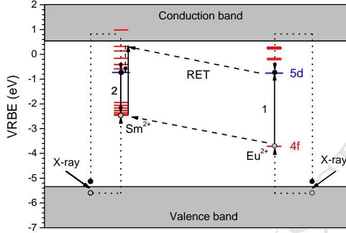
FIG. 7: Vacuum referred binding energy (VRBE) scheme for electrons in the 4f and 5d levels of  $\text{Sm}^{2+}$  and  $\text{Eu}^{2+}$  ions in a  $\text{SrI}_2$  host lattice, illustrating the resonant energy transfer (RET) process from  $\text{Eu}^{2+}$  to  $\text{Sm}^{2+}$ . The arrows are explained in the text.
