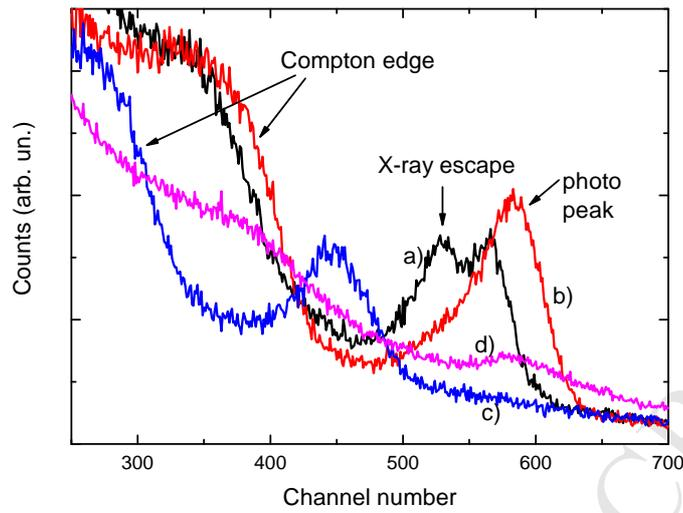
FIG. 3: Pulse-height spectra of a  $^{137}\text{Cs}$  source measured with the  $\text{SrI}_2:5\% \text{Eu}^{2+}$  samples doped with a) 0%, b) 0.05%, c) 0.2% and d) 0.5%  $\text{Sm}^{2+}$  at 250 K with an avalanche photodiode. Only the part around the Compton edge and 662 keV total absorption peak is shown.
