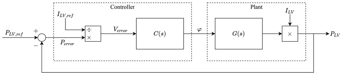
Figure 5.7: Schematic representation of the implemented closed loop system.
