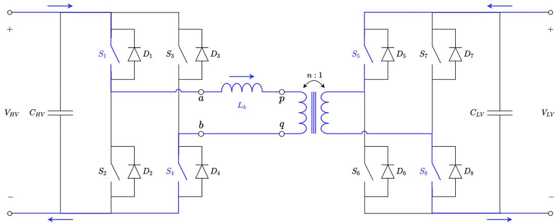
Figure 4.3: The current flow during period II.
