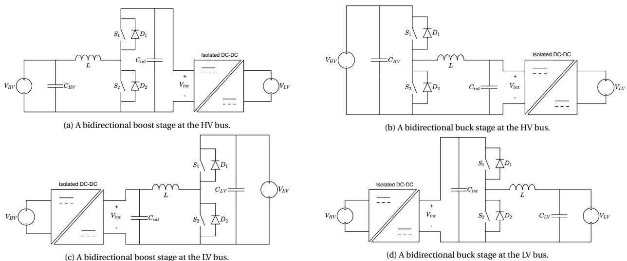
Figure 2.9: The four options for placement of bidirectional buck or boost converters.
