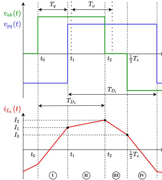
Figure 4.13: Zoomed half period waveforms for OTM-1 modulation.
