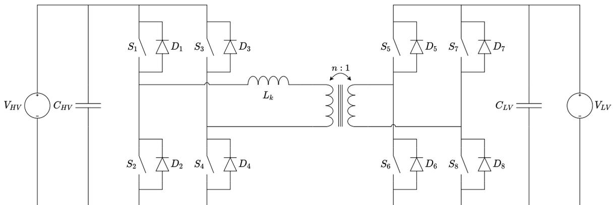
Figure 2.5: Schematic of a dual active bridge converter.
