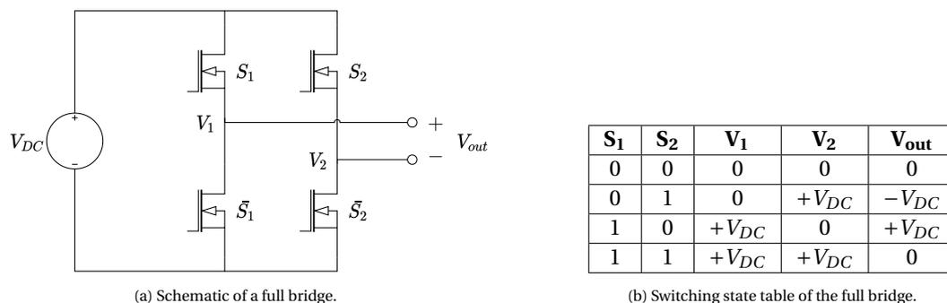
Figure 5.2: Schematic representation and switching table of a single switching leg.
