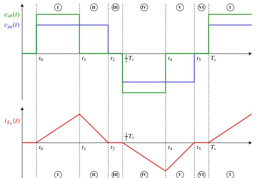
Figure 4.6: The waveforms of the DAB converter for TCM modulation with gate signals for the leading HV bridge.
