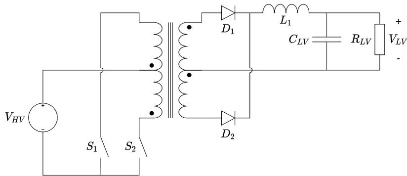
Figure 2.4: Schematic of a center tapped push-pull converter.
