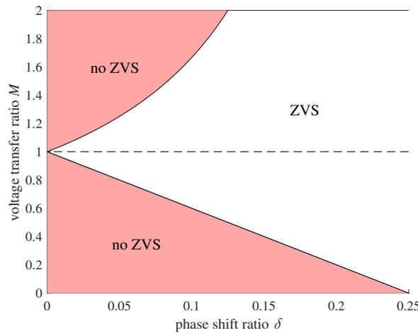
Figure 2.13: ZVS region for the ideal DAB converter.
