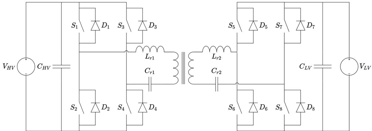
Figure 2.8: Schematic of a bidirectional CLLC resonant converter.
