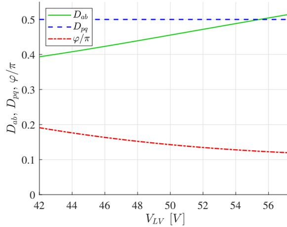
Figure 4.11: The calculated control variables for OTM for a full sweep over  $V_{LV}$  with  $V_{HV} = 346$  V.
