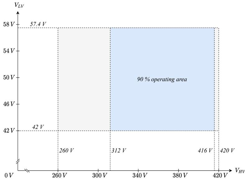
Figure 1.2: The 90 % use case operating window (blue) given within the full operating range (grey) for the bus voltages of the converter.
