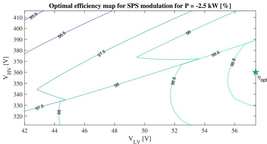
Figure 3.7: Contour plot showing the DAB power stage efficiency for the 90 % operating region for the design after trade-offs at a power of  $P = -2.5$  kW. The peak efficiency is depicted with a green star, which reaches 99.14 % for  $V_{HV} = 360$  V and  $V_{LV} = 57.4$  V.
