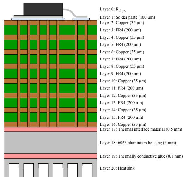
Figure C.1: One dimensional schematic representation of the thermal circuit for one MOSFET (not to scale).
