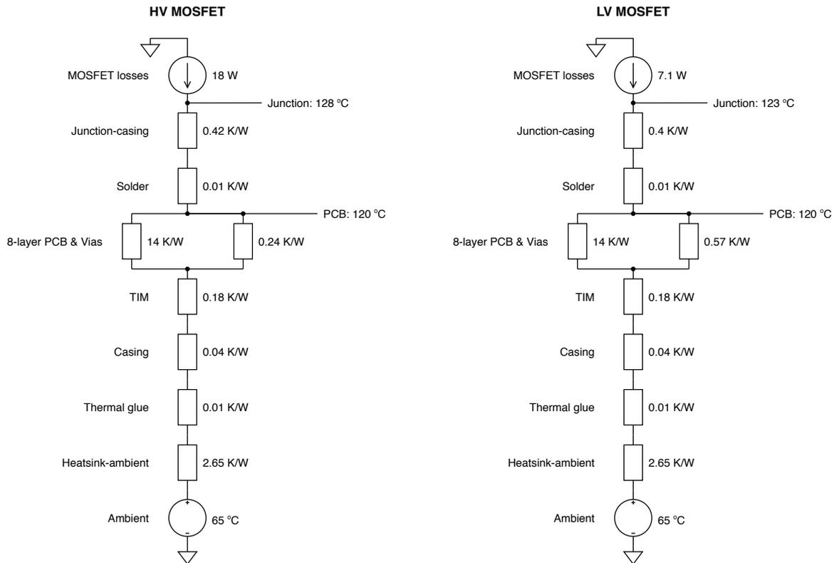
Figure C.2: Equivalent resistor network with thermal resistance per layer for one single HV and LV MOSFET.
