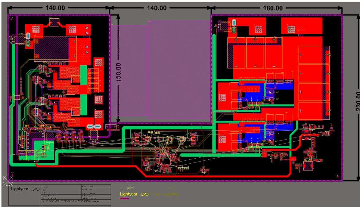
Figure C.3: Top view of the designed prototype PCB. The red planes are the top layer of the 8-layer PCB.
