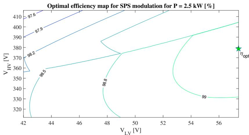
Figure 3.4: Contour plot showing the DAB power stage efficiency for the 90 % operating region with SPS modulation at a power of  $P = 2.5$  kW. The peak efficiency is depicted with a green star, which reaches 99.14 % for  $V_{HV} = 378.8$  V and  $V_{LV} = 57.4$  V.
