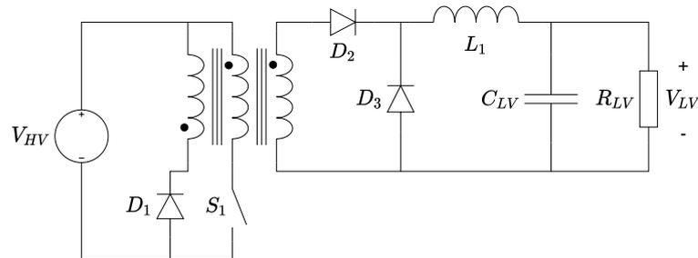
Figure 2.3: Schematic of a forward converter.
