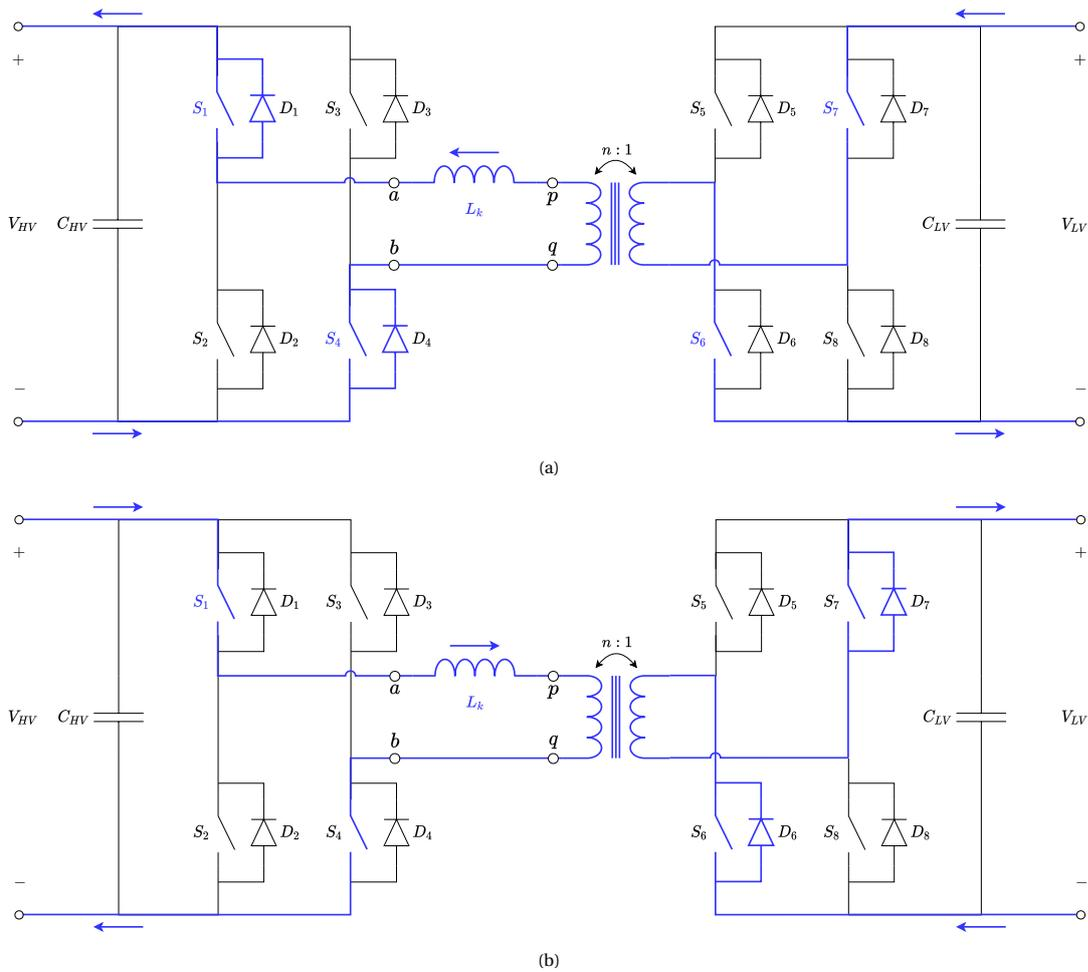
Figure 4.2: (a) The current flow, depicted with a blue conduction path, during period I for a negative inductor current and (b) for a positive inductor current.
