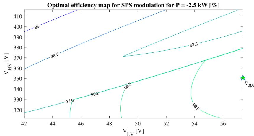
Figure 3.5: Contour plot showing the DAB power stage efficiency for the 90 % operating region with SPS modulation at a power of  $P = -2.5$  kW. The peak efficiency is depicted with a green star, which reaches 98.96 % for  $V_{HV} = 350.7$  V and  $V_{LV} = 57.4$  V.
