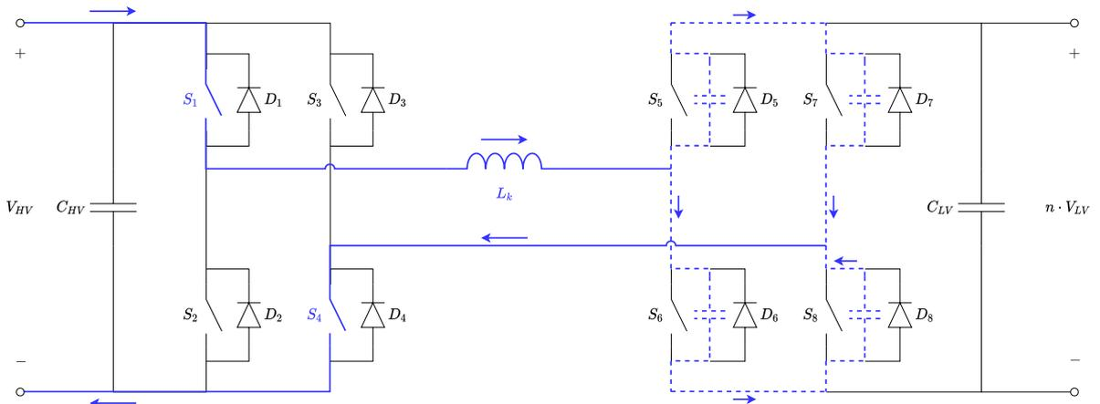
Figure 4.4: The current flow during the transition from period I to period II.
