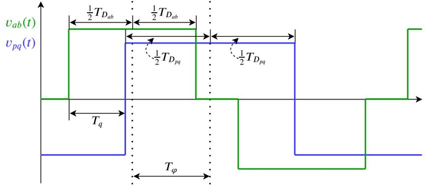
Figure 4.10: The definition of the phase shift time  $T_\varphi$  as used in further formulae, shown for OTM-1.
