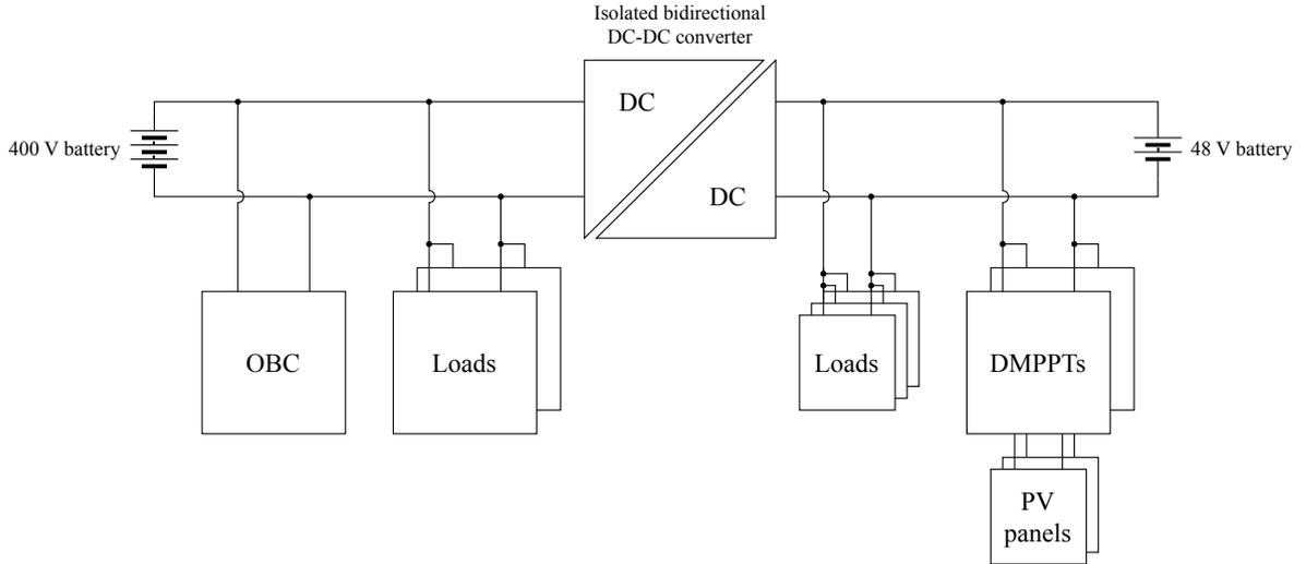
Figure 1.1: A simplified general system overview of the powertrain topology of the Lightyear One.
