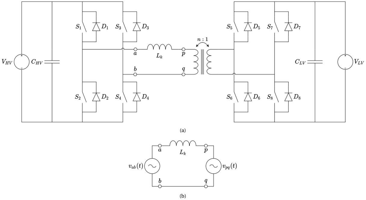
Figure 2.10: (a) The DAB converter with the ports of the HF transformer labelled. (b) Simplified schematic of the DAB converter.
