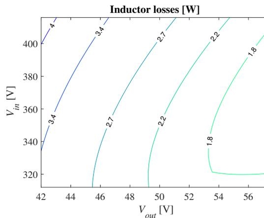
Figure 4.19: Inductor losses for the optimal DAB converter design according to table 4.7 at an output power of  $P_{LV} = 2.5$  kW.
