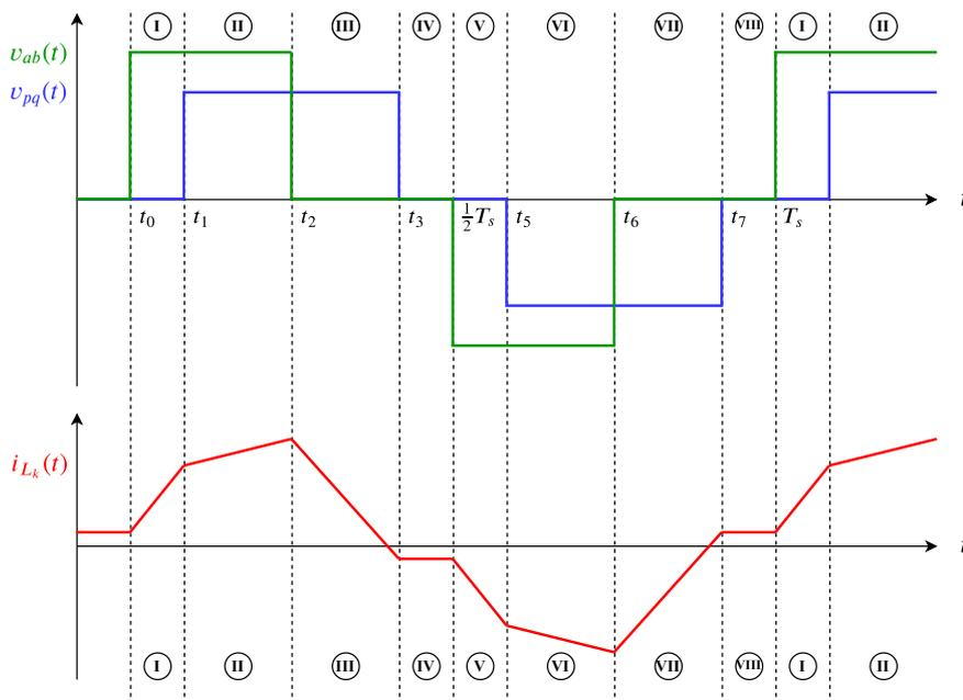
Figure 4.7: The waveforms of the DAB converter for TPS modulation.
