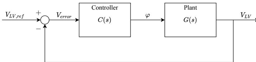
Figure 5.6: Schematic representation of a closed-loop controller implementation.
