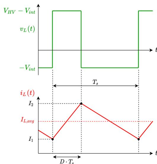
Figure 2.18: Ideal waveforms for buck operation of the bidirectional buck converter.
