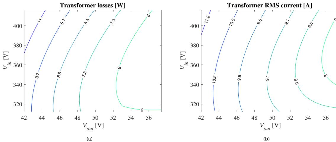
Figure 4.20: (a) Transformer losses for the optimal DAB converter design according to table 4.7 at a power of  $P_{LV} = 2.5$  kW and (b) the RMS current through the transformer for different operating points.
