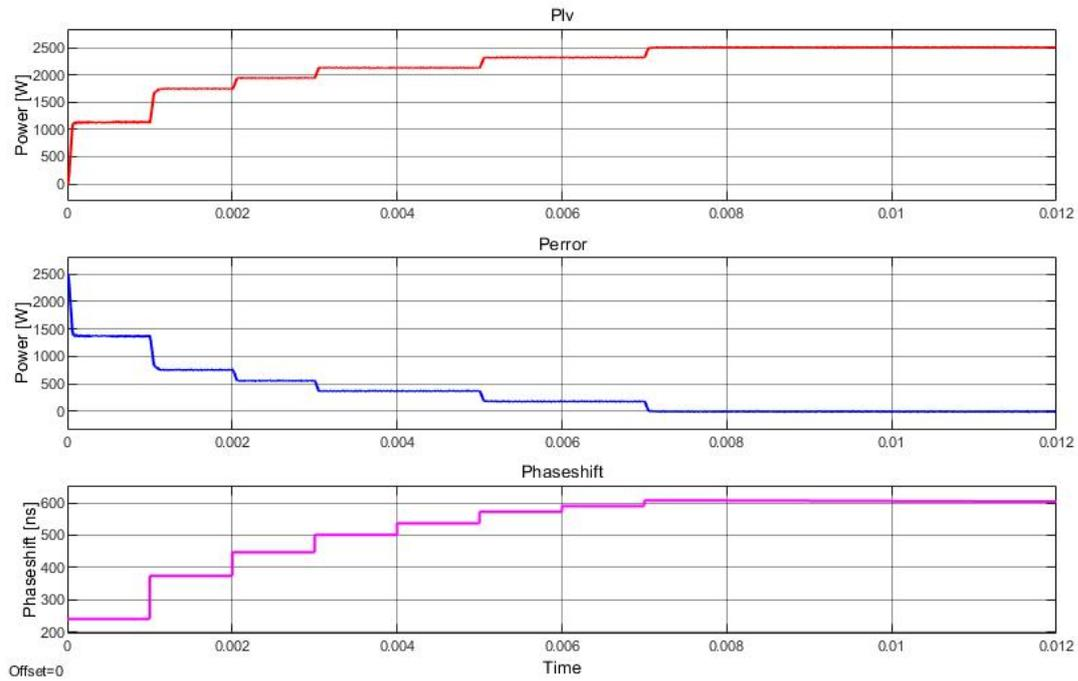
Figure 5.12: Start-up behavior of the DAB converter for  $P = 2.5$  kW,  $V_{HV} = 378$  V,  $V_{LV} = 50.4$  V,  $K_{p,pos} = 3 \cdot 10^{-3}$  and  $K_{i,pos} = 3$ .
