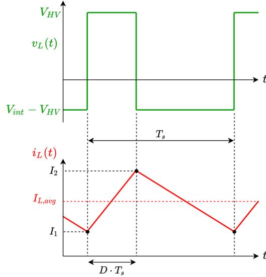
Figure 2.19: Ideal waveforms for boost operation of the bidirectional buck converter.
