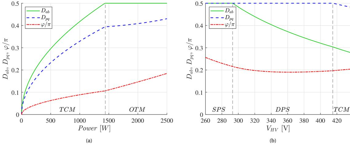
Figure 4.8: The control parameters of the optimal modulation scheme for (a) changing LV side power with  $V_{HV} = 260$  V and  $V_{LV} = 55$  V and (b) changing HV bus voltage with  $P_{LV} = 2.5$  kW. The DAB converter parameters are  $L_k = 25$   $\mu$ H,  $n = 6$  and  $f_s = 100$  kHz.
