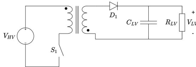
Figure 2.2: Schematic of a flyback converter.
