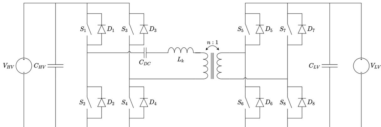
Figure 2.20: Schematic of a dual active bridge converter with added DC blocking capacitor.
