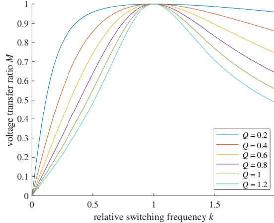
Figure 2.16: The voltage transfer ratio of the LLC converter in backward mode plotted against the relative switching frequency  $k$  for different power levels  $Q$ .
