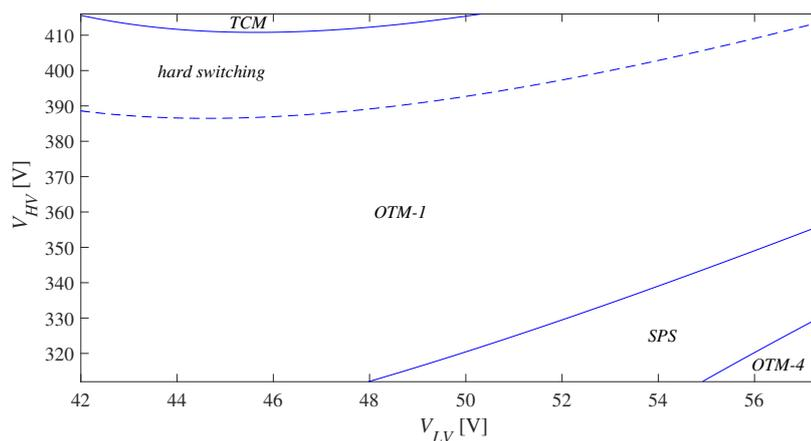
Figure 4.17: The boundaries of the different modulation schemes for  $P_{LV} = 2.5$  kW.
