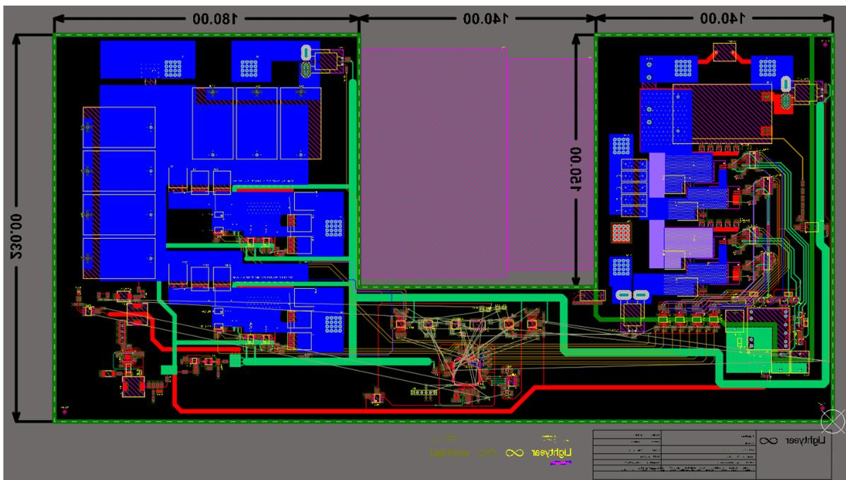
Figure C.4: Bottom view of the designed prototype PCB. The blue planes are the bottom layer of the 8-layer PCB.
