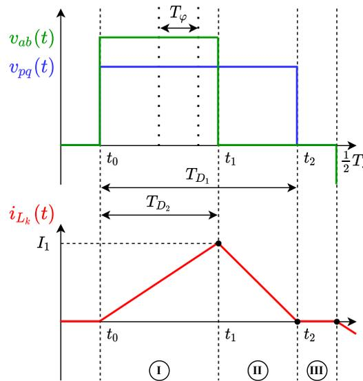
Figure 4.12: Zoomed half period waveforms for TCM modulation.
