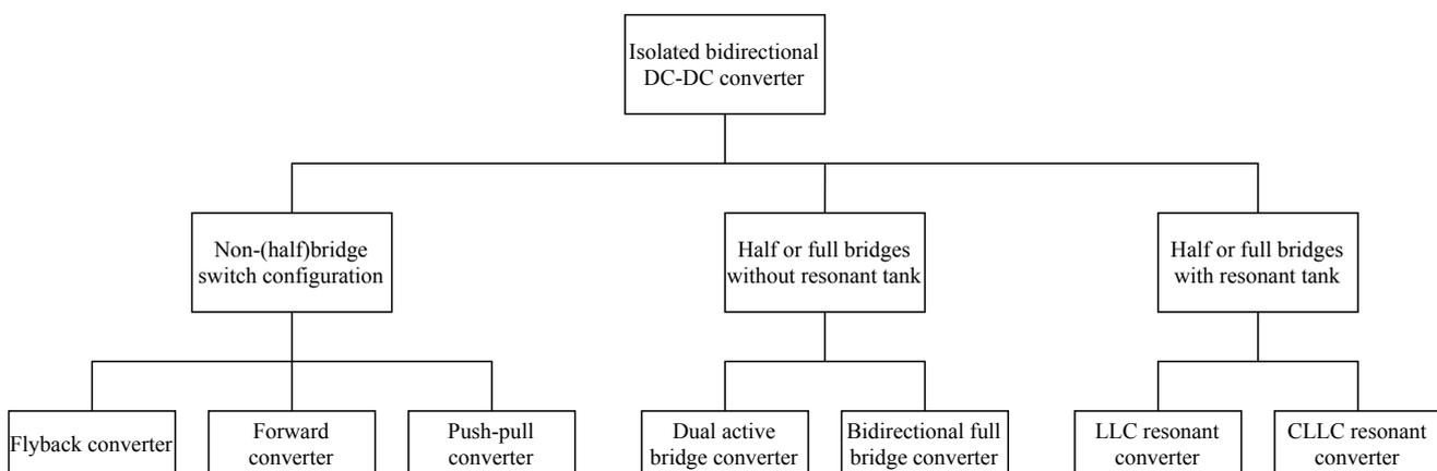
Figure 2.1: An overview of the different isolated bidirectional DC-DC converter topologies.
