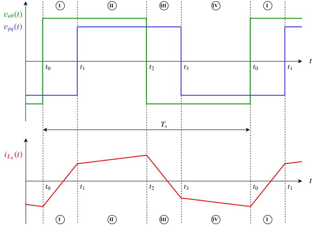
Figure 2.11: Ideal waveforms of the simplified DAB converter for SPS control in steady state.
