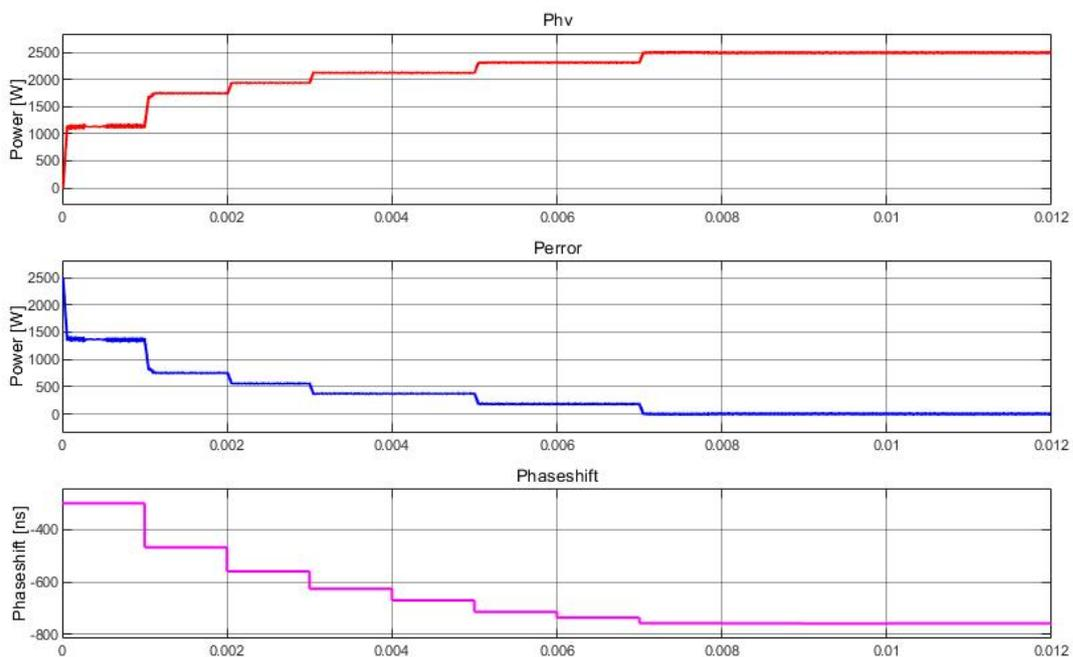
Figure 5.13: Start-up behavior of the DAB converter for  $P = -2.5$  kW,  $V_{HV} = 378$  V,  $V_{LV} = 50.4$  V,  $K_{p,neg} = 1 \cdot 10^{-4}$  and  $K_{i,neg} = 0.5$ .
