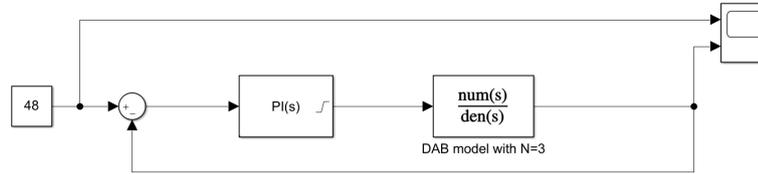
Figure 5.9: Implementation of the PI tuning loop.
