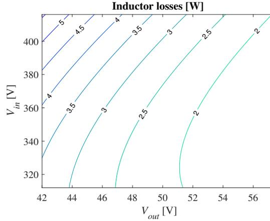
Figure 3.10: Inductor losses for the optimal DAB converter design at an output power of  $P_{LV} = 2.5$  kW.
