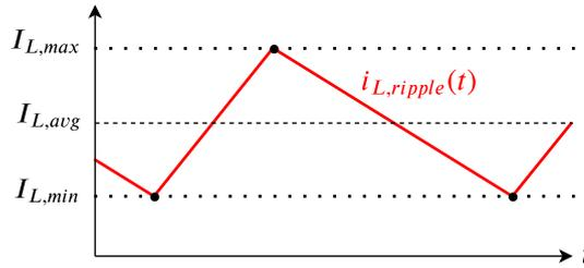
Figure A.1: Ideal inductor current waveform of a buck converter.
