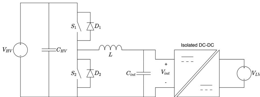
Figure 2.17: The schematic of the two stage converter with a buck stage at the HV side.
