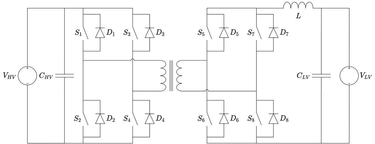
Figure 2.6: Schematic of a bidirectional current-fed full bridge converter.
