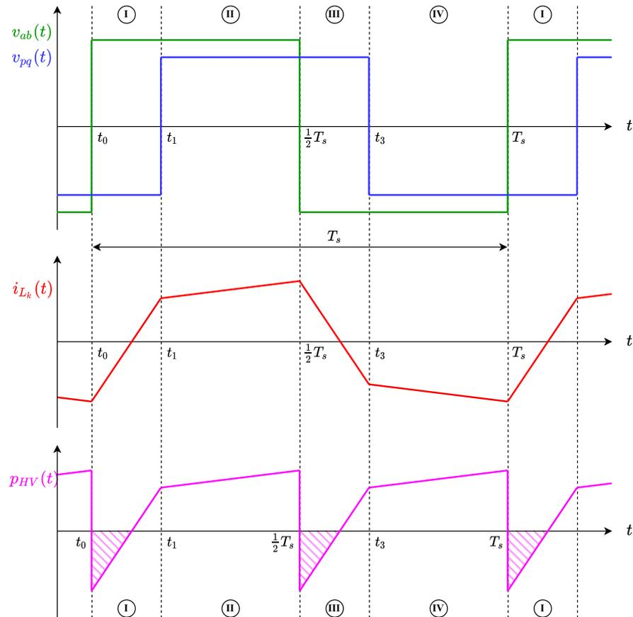
Figure 4.1: Region definition of the waveforms of the simplified DAB converter using SPS modulation, including converter power as supplied by the HV bus.
