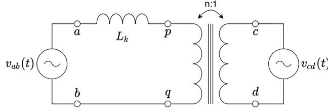
Figure 5.3: Simplified circuit of the DAB converter.
