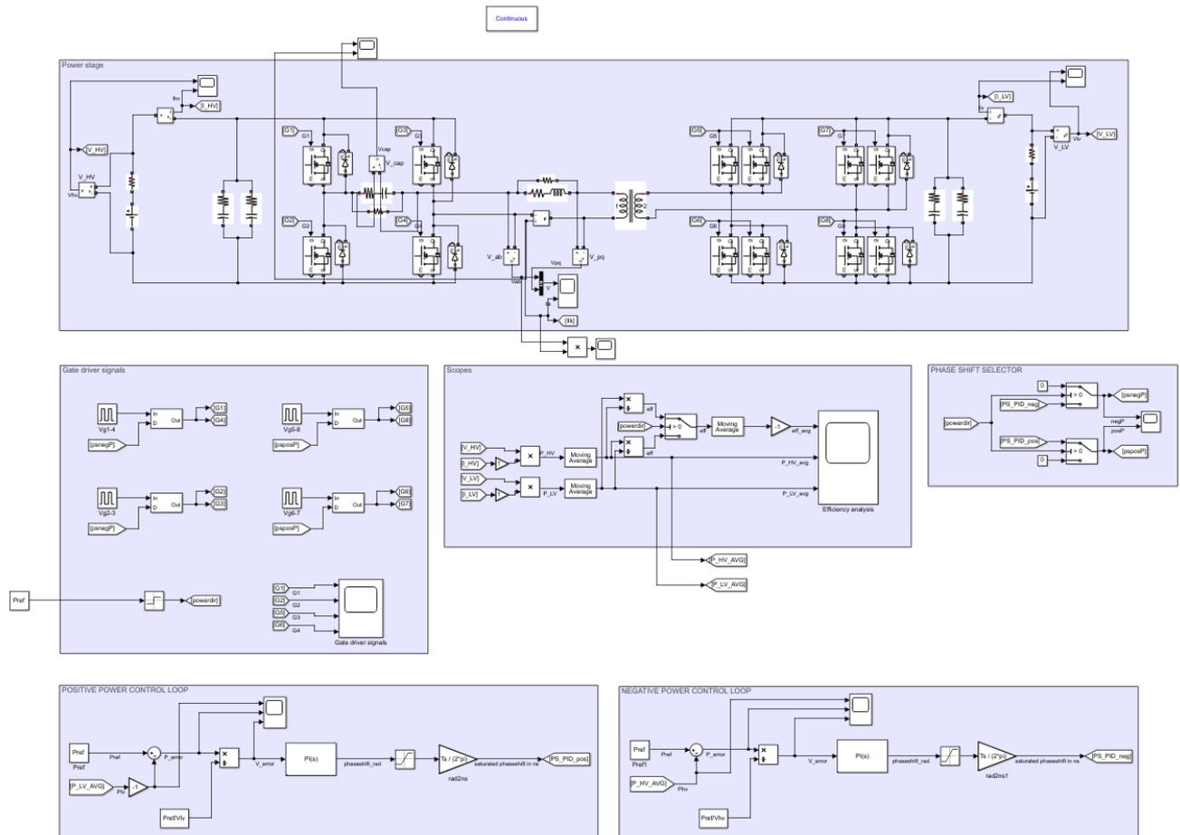
Figure 5.11: Implemented Simulink model of the designed DAB converter with control loop.
