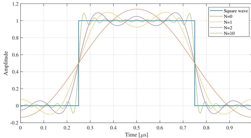
Figure 5.4: Ideal square wave signal approached by Fourier series with different number of harmonics.
