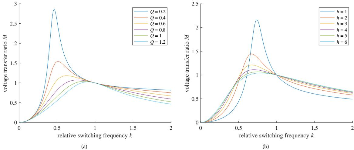
Figure 2.15: The voltage transfer ratio of the LLC converter plotted against the relative switching frequency  $k$  for (a) different power levels  $Q$  with  $h = 4$  and (b) different inductor ratios  $h$  with  $Q = 0.7$ .
