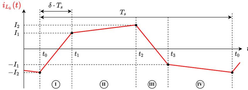
Figure 2.12: Zoomed ideal inductor current waveform of the simplified DAB converter for SPS control in steady state.
