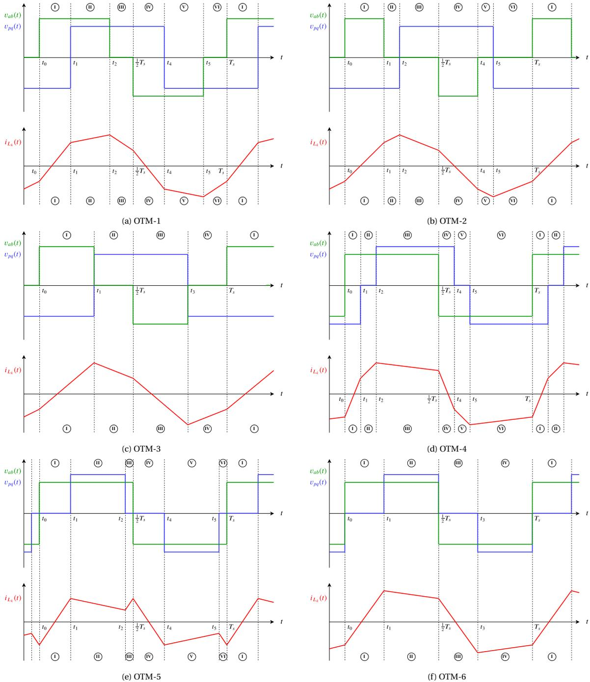
Figure 4.9: Schematic representation of different waveform options for OTM modulation for positive power flow, with a leading HV bridge. For (a)-(c) it holds that  $\bar{V}_{ab} > \bar{V}_{pq}$ , resulting in  $D_{pq} = 0.5$ . For (d)-(f) it can be seen that  $\bar{V}_{ab} \leq \bar{V}_{pq}$ , resulting in  $D_{ab} = 0.5$ .
