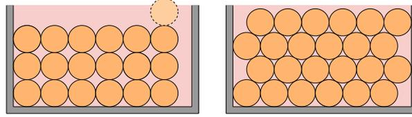
Figure B.2: Cross section view of the winding area utilization, showing the conservative method on the left and the realistic method on the right. The orange circles are the conductors, the grey bounds the bobbin walls and the red background shows the unused area.
