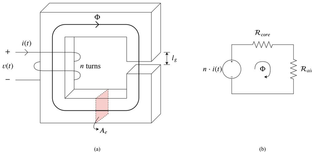
Figure B.1: Magnetic diagram for an inductor with air gap depicted as (a) a structure and (b) an equivalent circuit.  $\Phi$  is the flux through the structure and  $\mathcal{R}$  the reluctance of the magnetic circuit.
