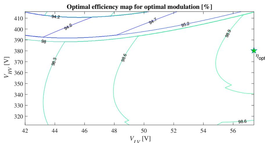
Figure 4.15: Contour plot showing the DAB power stage efficiency with optimal modulation at an output power of  $P_{LV} = 2.5 \text{ kW}$ . The peak efficiency is depicted with a green star, which reaches 99.32 % for  $V_{HV} = 375.2 \text{ V}$  and  $V_{LV} = 57.4 \text{ V}$  over the 90 % operating region.
