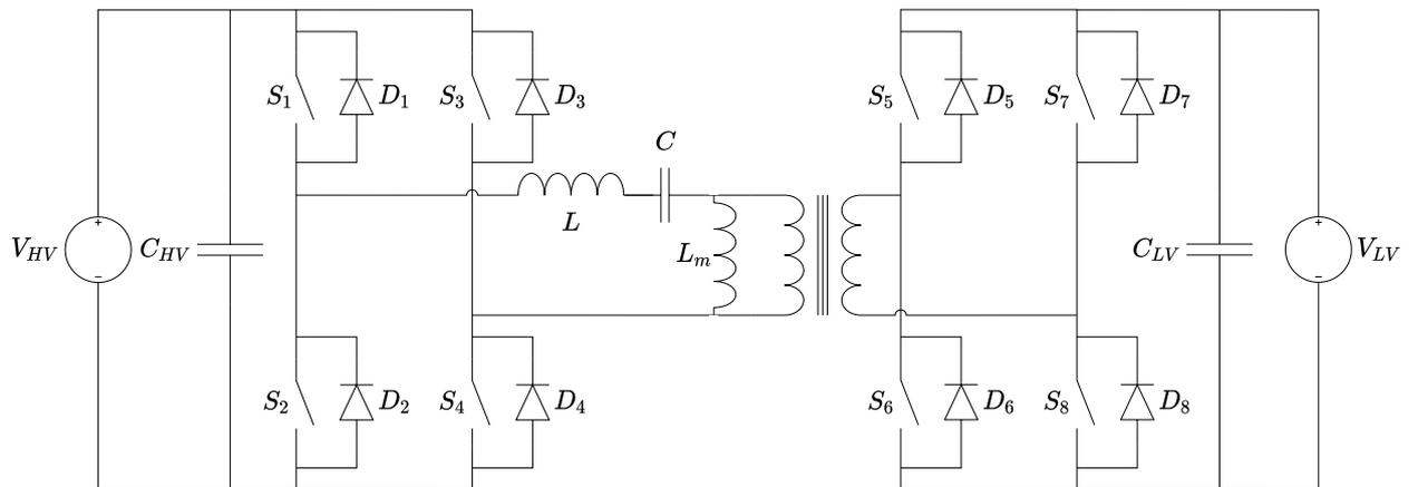
Figure 2.7: Schematic of a bidirectional LLC resonant converter.
