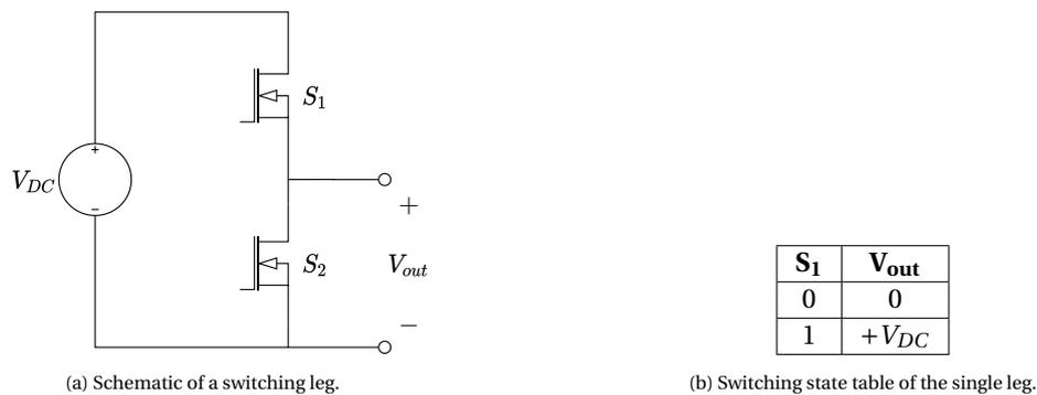
Figure 5.1: Schematic representation and switching table of a single switching leg.
