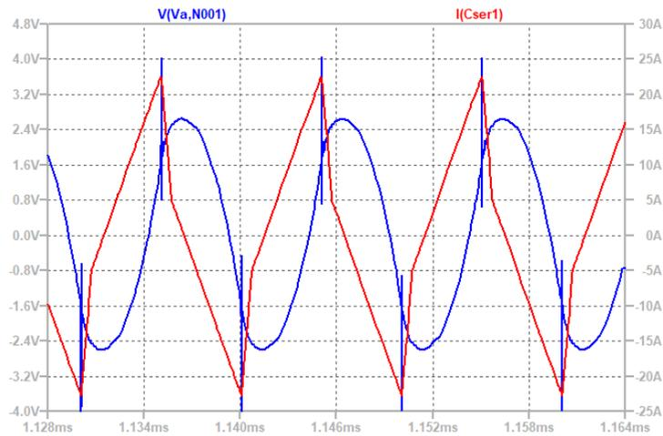
Figure 3.3: LTspice simulation waveforms of the series DC blocking capacitor in steady state for  $V_{HV} = 437$  V and  $V_{LV} = 42$  V with  $P_{LV} = 2500$  W. The blue trace is the capacitor voltage and the red trace is the (total) capacitor current.
