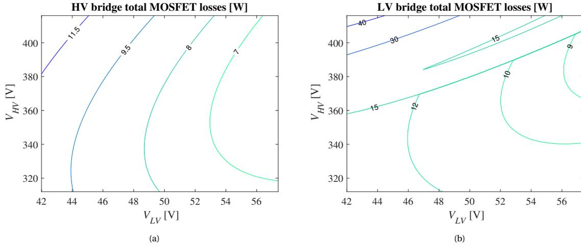
Figure 3.8: MOSFET losses for the optimal DAB converter design according to table 3.7 at an output power of  $P_{LV} = 2.5$  kW. (a) shows the total HV bridge losses and (b) the total LV bridge losses.
