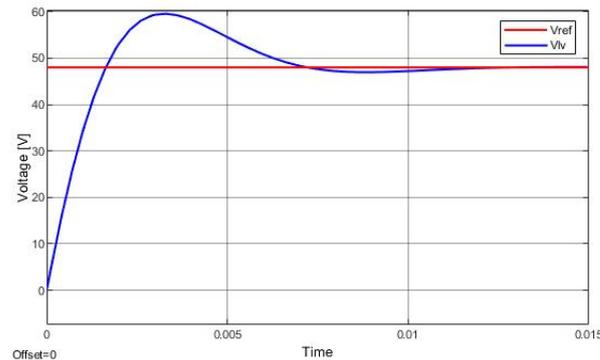
Figure 5.10: Start-up response of the converter model for positive power transfer.
