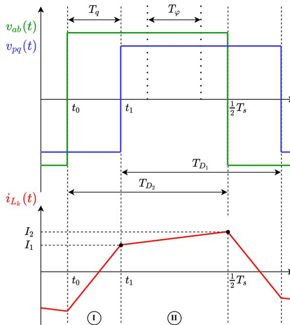
Figure 4.14: Zoomed half period waveforms for SPS-1 modulation.
