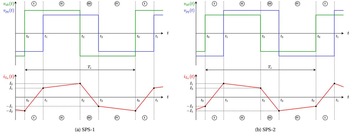
Figure 3.1: The two possible waveforms for SPS modulation. (a) with  $V_{HV} > V_{LV}$  and (b) with  $V_{HV} < V_{LV}$ .
