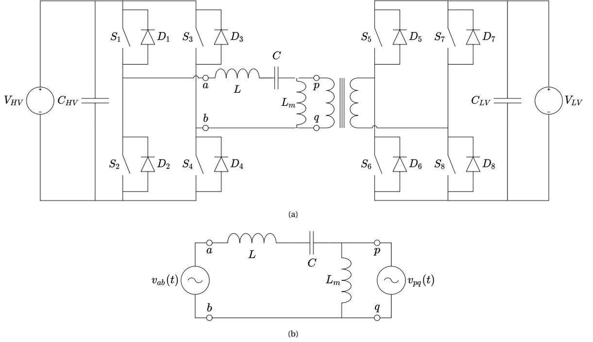
Figure 2.14: (a) The LLC converter with the ports of the HF transformer labelled. (b) Simplified schematic of the LLC converter.
