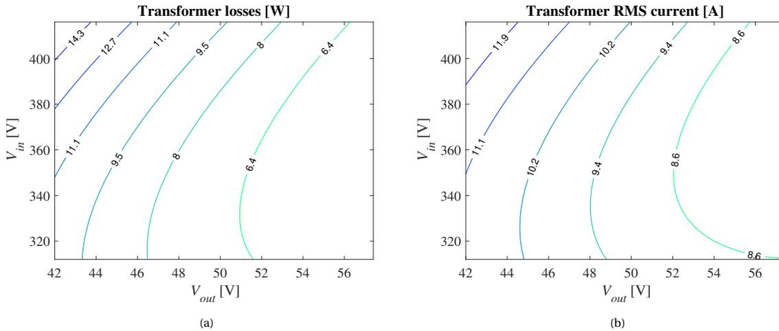
Figure 3.11: (a) Transformer losses for the optimal DAB converter design according to table 3.7 at a power of  $P_{LV} = 2.5$  kW and (b) the RMS current through the transformer for different operating points.
