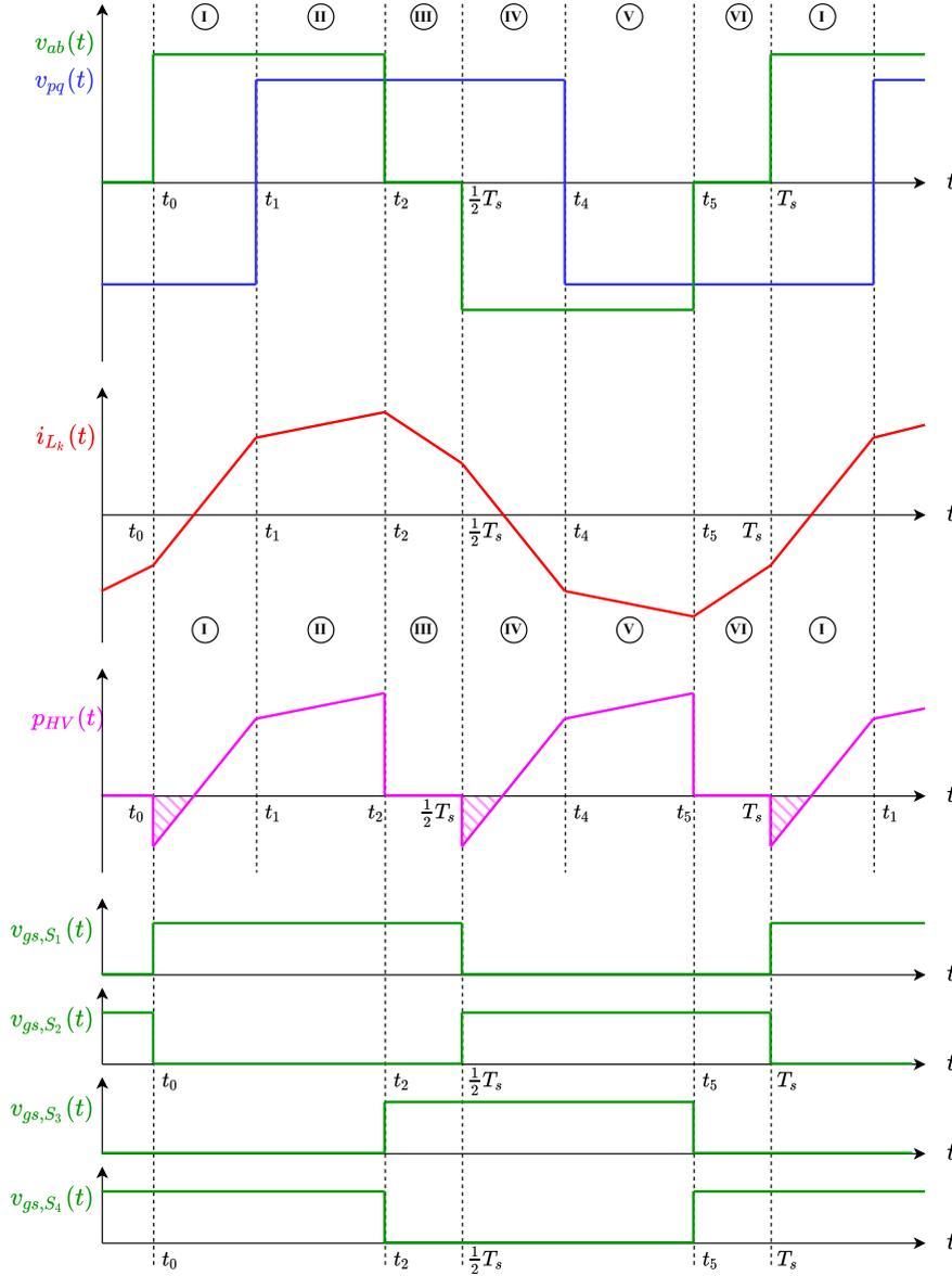
Figure 4.5: The waveforms of the DAB converter for EPS modulation, including HV bus power and gate signals for the leading HV bridge.
