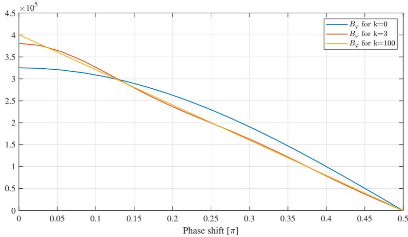
Figure 5.5: Influence of the higher order harmonics on the  $B_\varphi$  term for changing phase shift  $\varphi$ .
