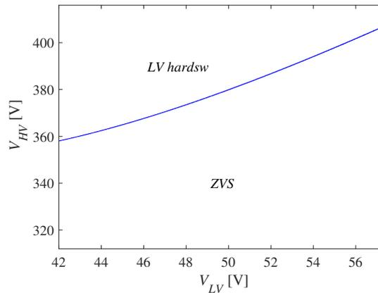
Figure 3.9: Hard switching region, depicted as LVhardsw, of the LV full bridge at a power of  $P = 2.5$  kW.
