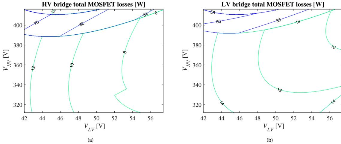
Figure 4.18: Switch losses for the optimal DAB converter design according to table 4.7 at an output power of  $P_{LV} = 2.5$  kW. (a) shows the total HV bridge losses and (b) the total LV bridge losses.
