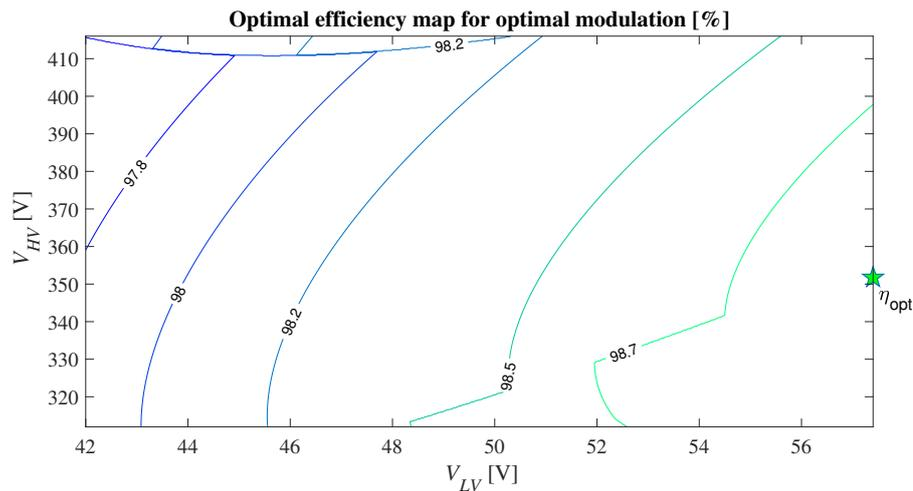
Figure 4.16: Contour plot showing the DAB power stage efficiency with optimal modulation at an output power of  $P_{LV} = -2.5$  kW. The peak efficiency is depicted with a green star, which reaches 98.92 % for  $V_{HV} = 351.7$  V and  $V_{LV} = 57.4$  V over the 90 % operating region.
