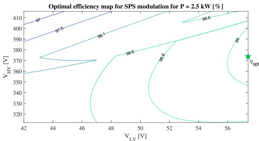
Figure 3.6: Contour plot showing the DAB power stage efficiency for the 90 % operating region for the design after trade-offs at a power of  $P = 2.5$  kW. The peak efficiency is depicted with a green star, which reaches 99.14 % for  $V_{HV} = 371.7$  V and  $V_{LV} = 57.4$  V.
