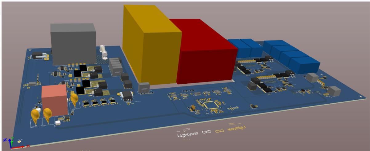
Figure C.5: Three-dimensional view of the designed prototype PCB. The yellow block is the inductor placeholder, the red block the transformer placeholder.
