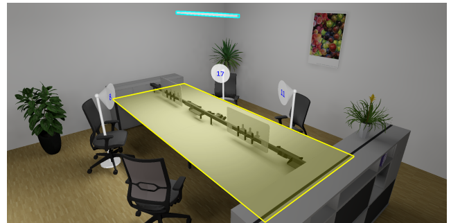
Fig. 2. A measuring surface on the desktop, and glare probes (simulating a person’s field of view while working on this desk) are used to gather illumination information, such as the average illuminance and the uniformity on an area, or if a person is likely to be blinded. Depending on the semantics, the target values of the measurement objects are set according to industry norms. Only designs in which all of these target values are reached are considered valid. To fully support linking and brushing in case of occlusions, outline-based highlighting enhancements and semi-transparent area overlays are rendered without depth-testing.
