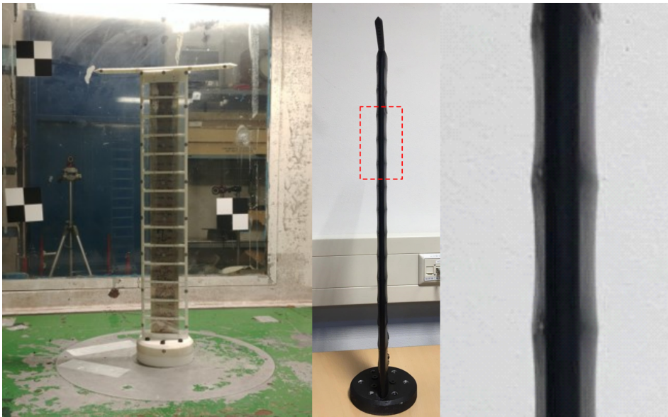
Figure 1: Pazy Wing in wind tunnel at Technion (left) [1]. Outer surface of the Pazy Wing from TU Delft in undeflected jig-shape with close up highlighting the sagging skin (foil cover) between the ribs.
