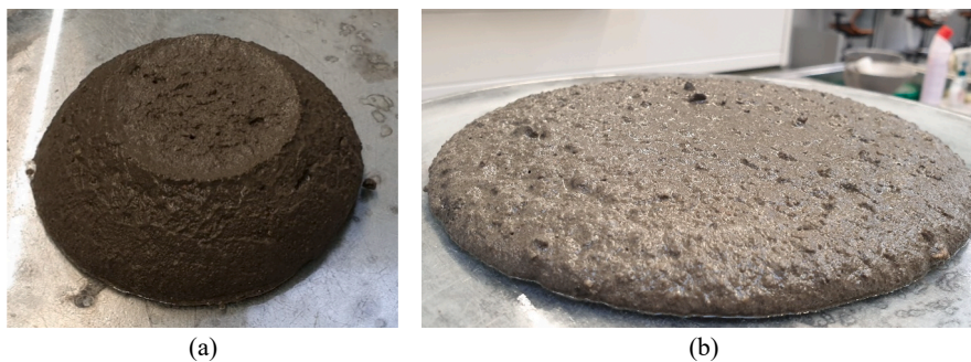
Fig. 5. Flow after 15 S, mortars with 25 wt% replacement, fRCA C, (a) SP: 0.2 wt% by cement (flow: 138 mm), (b) SP: 0.4 wt% by cement (flow: 187.5 mm).
