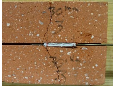
B (Full debonding with diagonal cracks)
