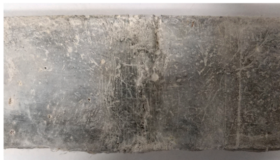
Fig. 5. The sample appearance after three-point bending test (the surface which contacts with two supporting points during bending).
