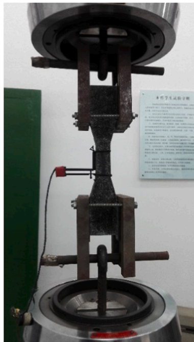
Fig. 3. The setup of uniaxial tensile test.
