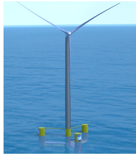
Figure 2.2: VoltornUS-S floater and IEA 15 MW reference turbine [Retrieved from [7]]
