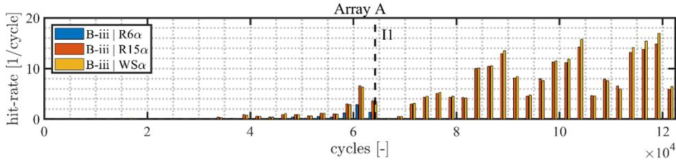
**Fig. 4.** Load-cycle normalised activity during the natural degradation test with the bogie wheel set-up (B-iii) recorded by the sensor node  $D_A$  near GS-2.
