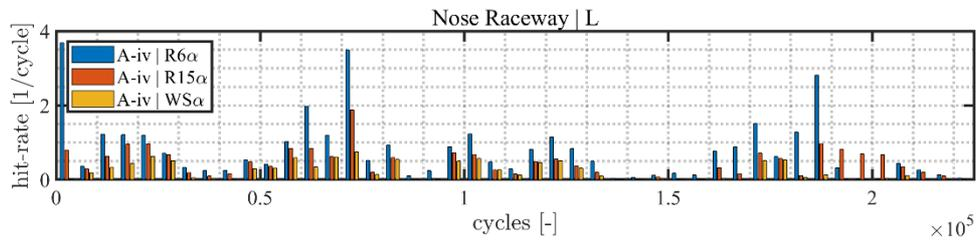
**Fig. 5.** Load-cycle normalised activity during the natural degradation test with the slew segment set-up (A-iv) recorded by the nose raceway sensor node.
