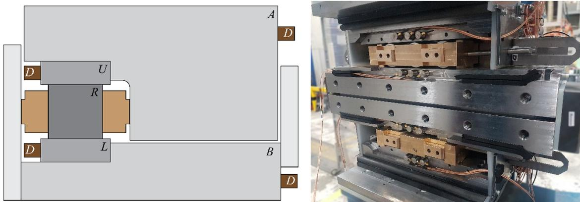
**Fig. 1.** Schematic overview of the upper chamber the of the slew segment test set-up (left), and a picture of the test set-up (right). Labels in the cross-section indicate the roller (*R*), nose raceway (*L*), support raceway (*U*), nose substructure (*B*), support substructure (*A*), and sensor nodes (*D*).
