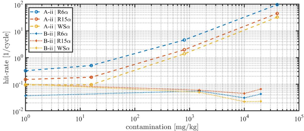
**Fig. 3.** Overview of load-cycle normalised activity for artificial contamination tests with the slew segment set-up (A-ii) and the bogie wheel set-up (B-ii). The baseline activity measurements for both set-ups (A-i, B-i) are plotted at  $10^0$  mg/kg contamination.
