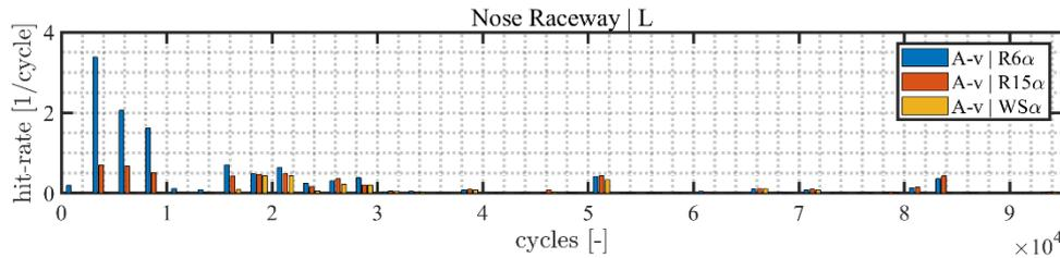
**Fig. 6.** Load-cycle normalised activity during the continued natural degradation test with the slew segment set-up (A-v) recorded by the nose raceway sensor node.
