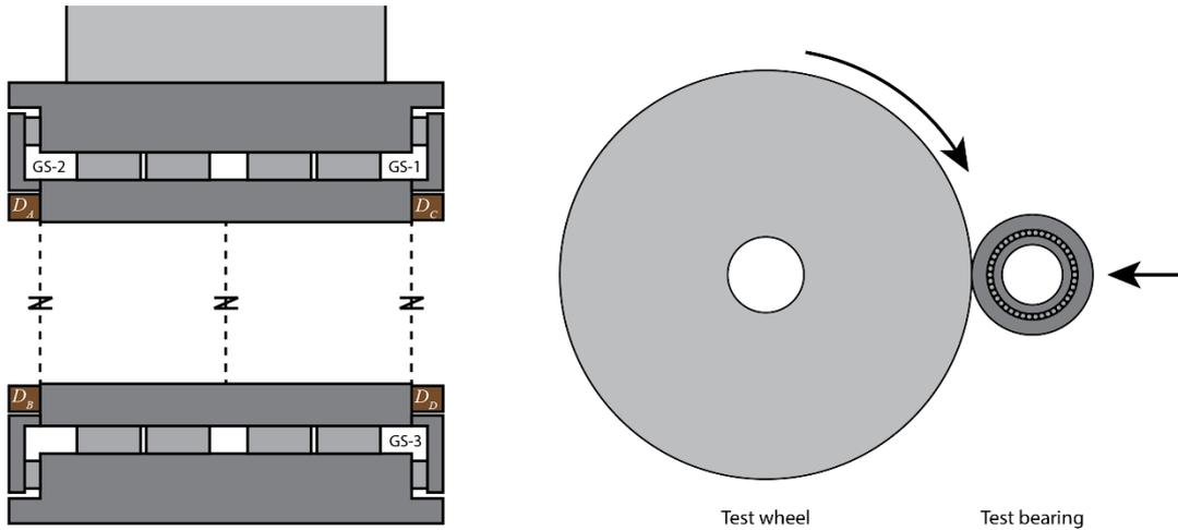
**Fig. 2.** Schematic overview of bogie wheel bearing (left), and testing arrangement (right). Labels in the cross-section indicate the sensor nodes ( $D_x$ ) and grease sampling locations (GS- $n$ ).
