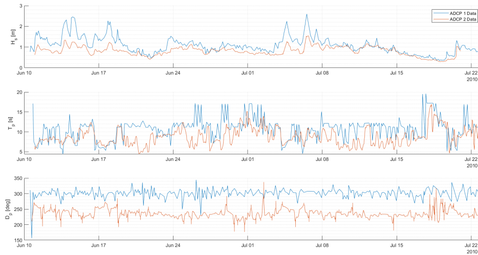
Figure 14: Nearshore significant wave height, peak period and peak direction results measured from two ADCP locations near the Port of San Antonio.
