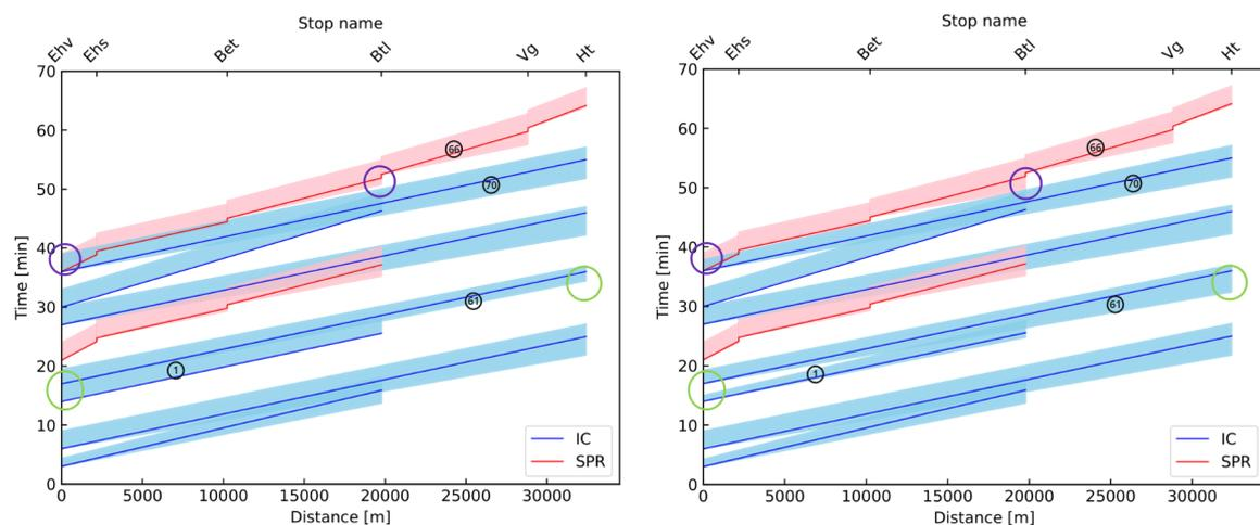
(a) Flexible train paths from Ehv to Ht without initial delay with  $e^{f,dep}$  is 1.1
