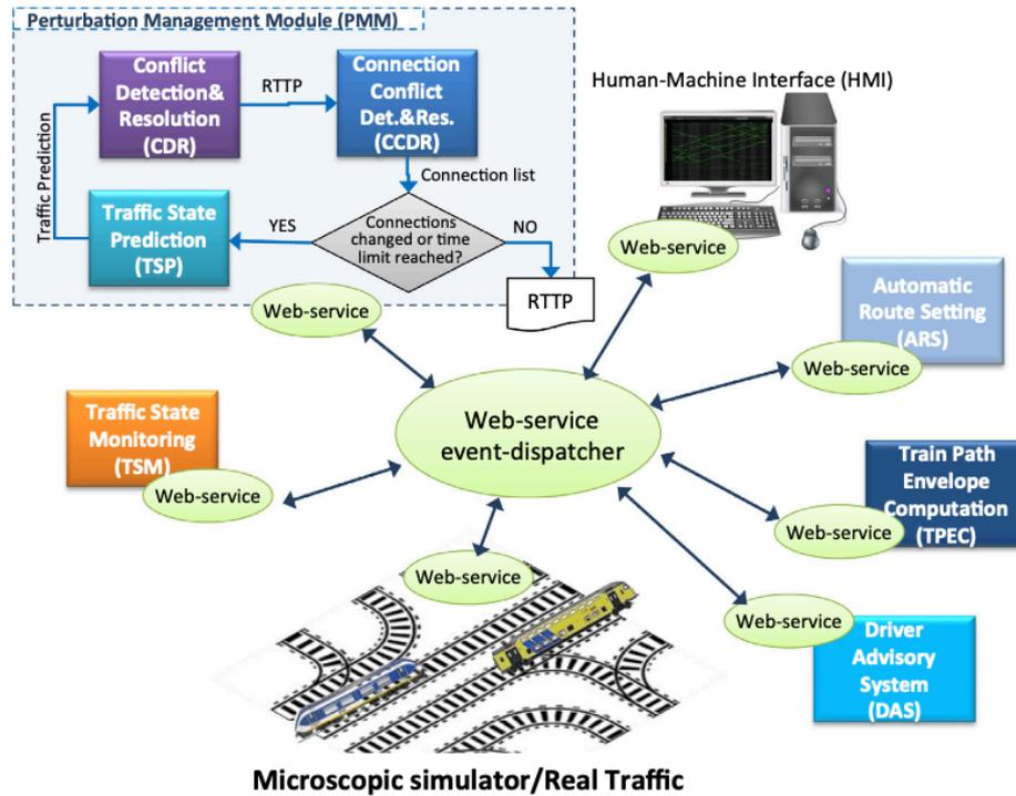
Figure 2.2: The ON-TIME framework for the real-time management of railway traffic perturbations (Quaglietta et al., 2016)
