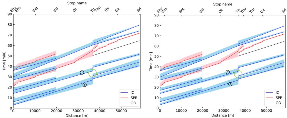
(a) Flexible train paths from Ehv to Bd without initial delay with  $e^{f, dep}$  is 1.1 (b) Flexible train paths from Ehv to Bd without initial delay with  $e^{f, dep}$  is 0.9
