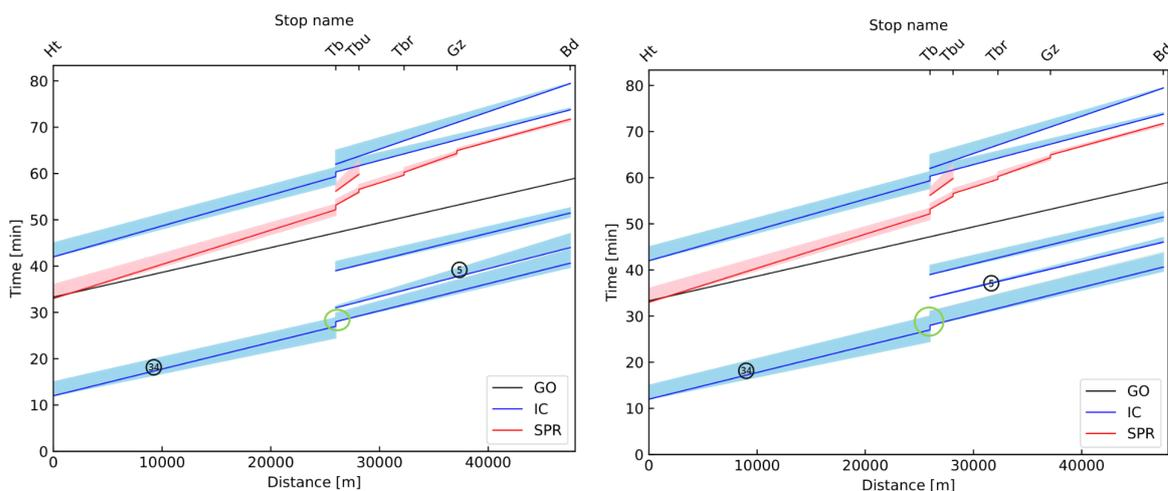
(a) Flexible train paths from Ht to Bd with 300 s initial delays added to train 5 (b) Flexible train paths from Ht to Bd with 600 s initial delays added to train 5
