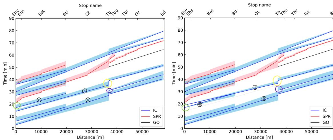
(a) Flexible train paths from Ehv to Bd with 0 s initial delay added to trains in the network
