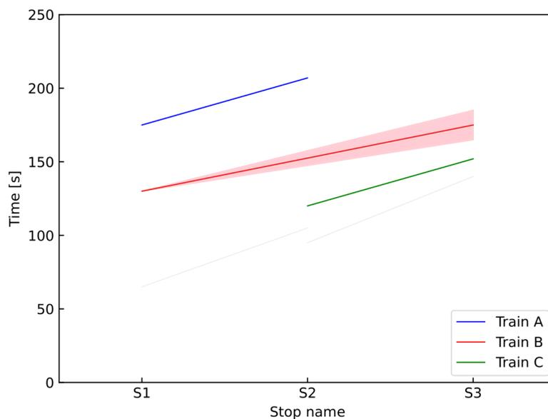
Figure 3.10: The train paths of three trains with initial delays
