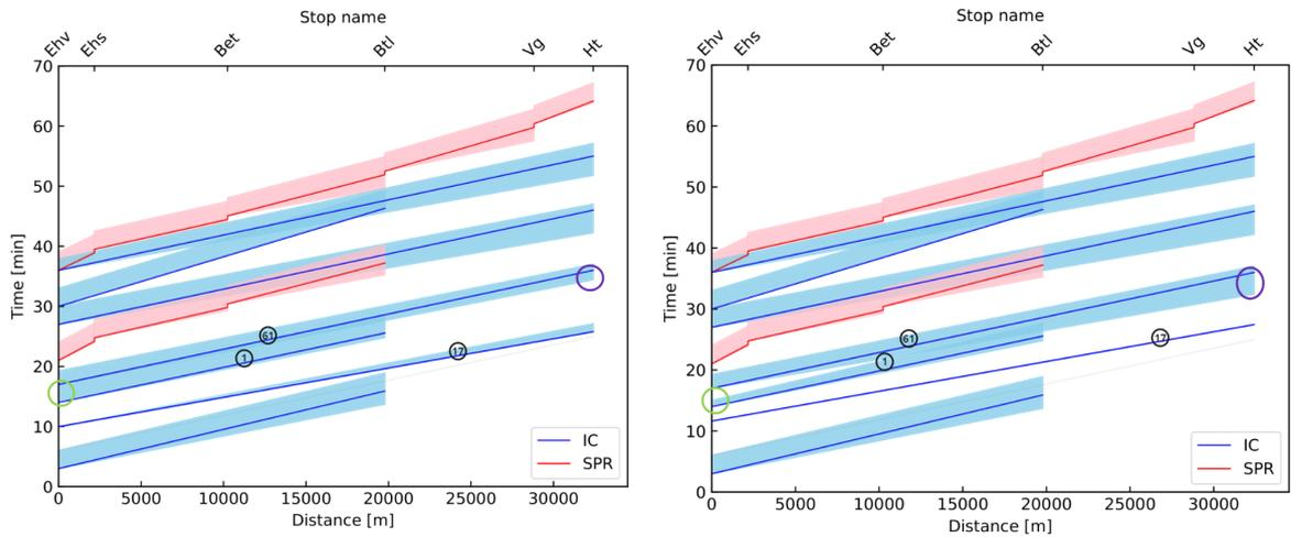
(a) Flexible train paths from Ehv to Ht with 400 s initial delays added to train 17 (b) Flexible train paths from Ehv to Ht with 500 s initial delays added to train 17
