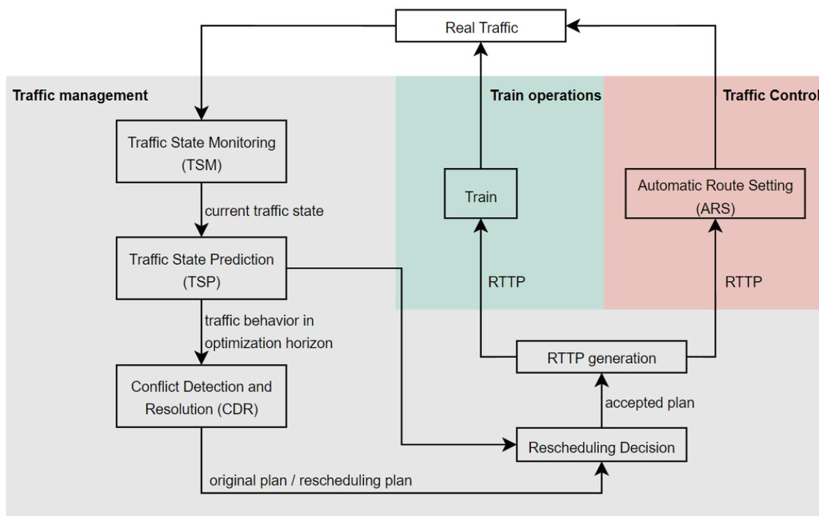
Figure 3.1: Framework for real-time railway operations
