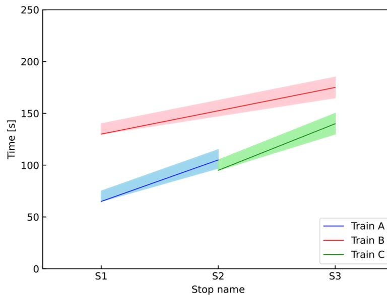
Figure 3.8: The train paths of three trains without initial delays
