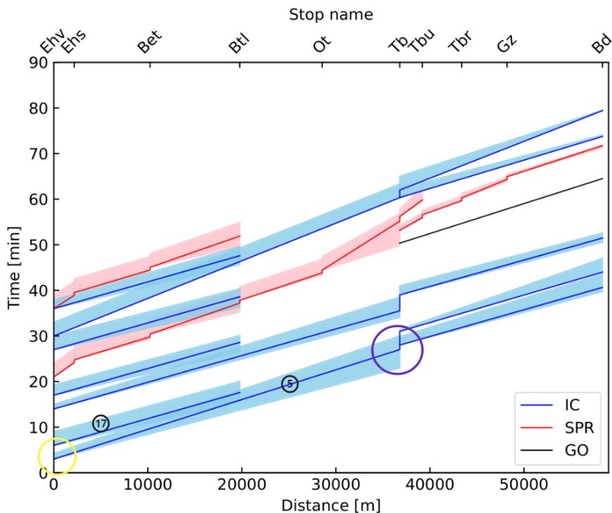
Figure 4.2: Train paths from Ehv to Bd without initial delays
