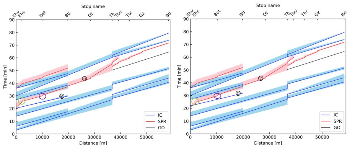
(a) Flexible train paths from Ehv to Bd with 500 s initial delays added to train 61 (b) Flexible train paths from Ehv to Bd with 600 s initial delays added to train 61
