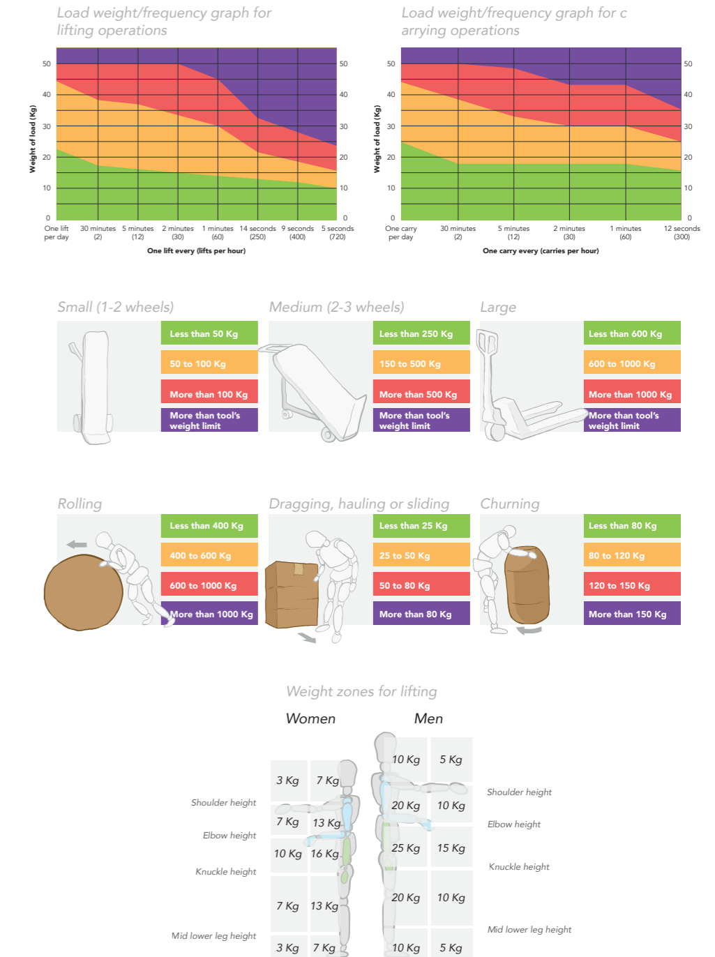
Figure 3: Manual handling load weight limits, original visuals by HSE
