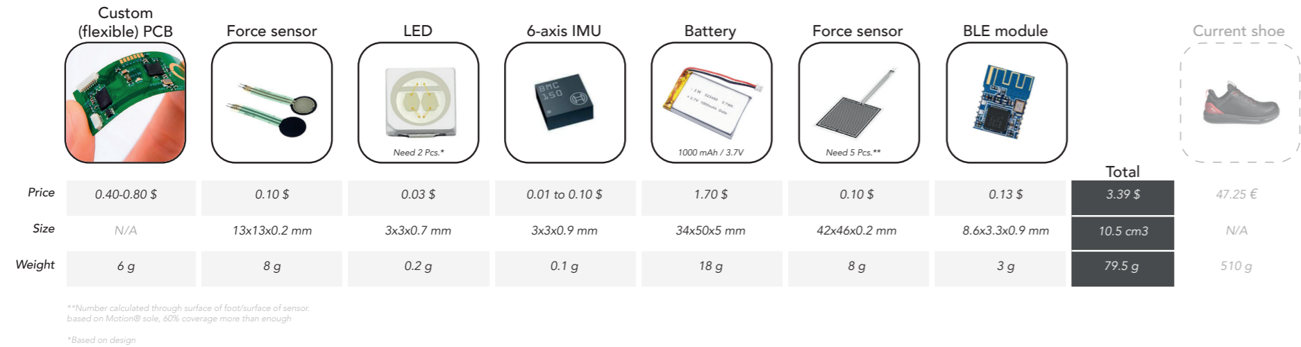
Figure 21: Overview of needed components their weight, size and price, per shoe.
