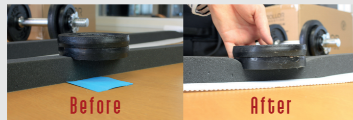
Figure 27 This figure shows the loss in pressure resistance in the foam rail after being rolled up tightly for four weeks. More results of the rail test are found in the appendices.
