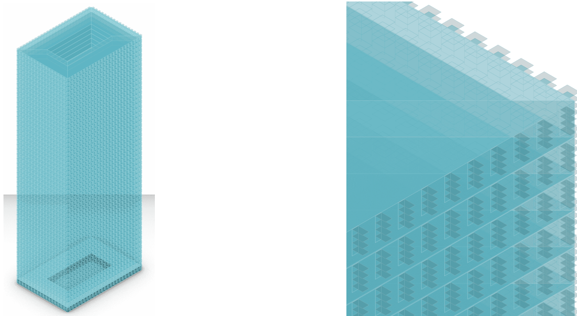
Figure A.30: Visualization of a design solution with low wwr and four horizontal louvres of 0.9 m depth.
