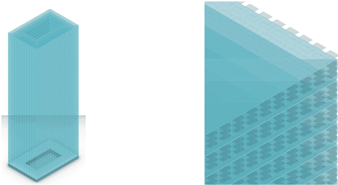
Figure A.31: Visualization of a design solution with high wwr and three horizontal louvres of 0.9 m depth.
