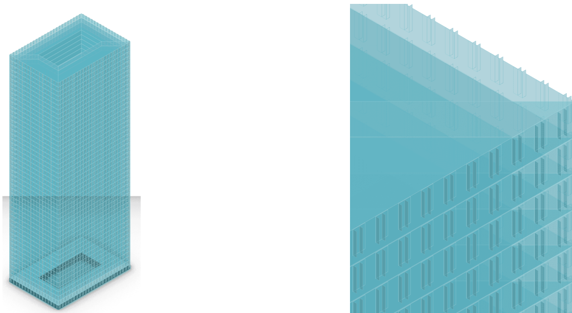
Figure A.32: Visualization of a design solution with low wwr and two vertical louvres of 0.3 m depth.
