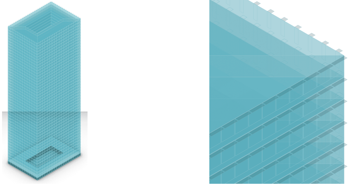
Figure A.33: Visualization of a design solution with low wwr and one horizontal overhang of 0.5 m depth.
