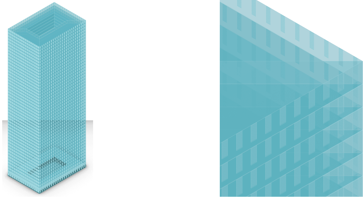
Figure A.29: Visualization of a design solutions with low wwr and internal blinds.
