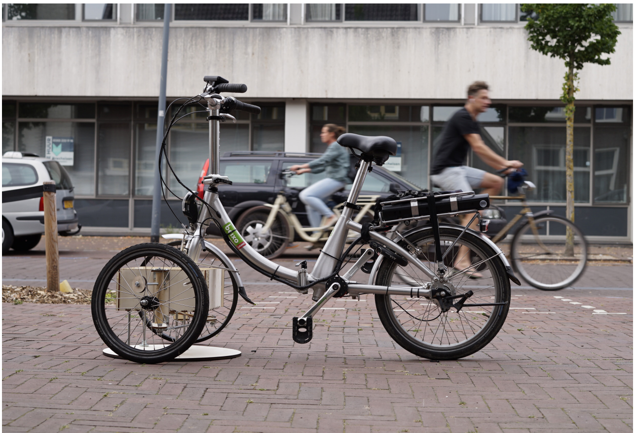
figure 69: 16 inch front wheels and 20 inch rear wheel
