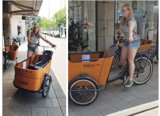
figure 48: The Babboe Curve is uncomfortable to steer
