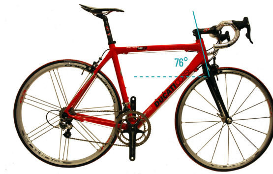
figure 71: A racing bike has a steep head tube
