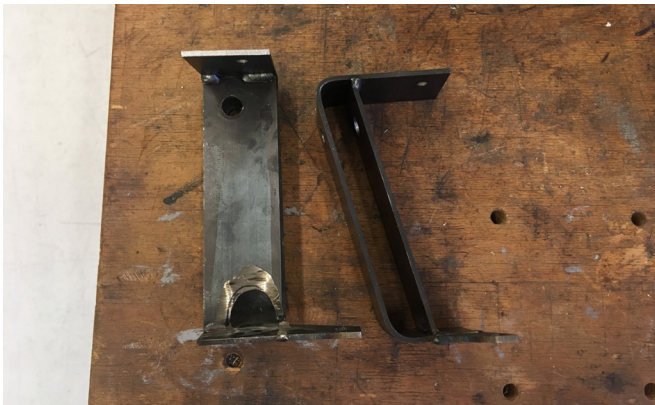
figure 196: The pivot arms were made by bending steel sheets and welding. The second plate, which functions as reinforcement touched the kingpin and thus part of it needed to be cut away.
