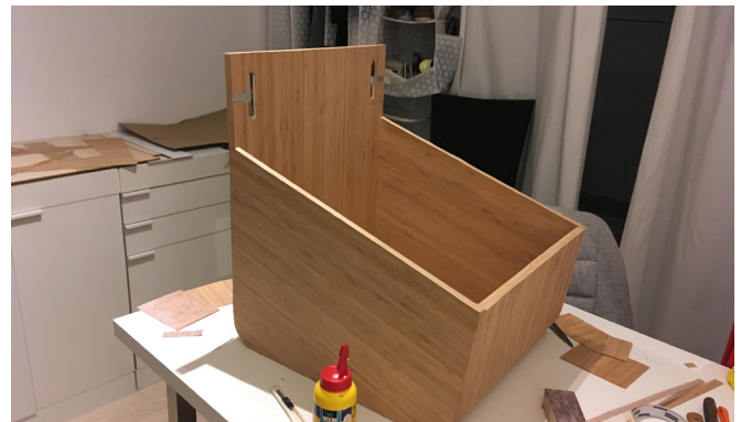
figure 176: In the prototype the sides are covered with bamboo veneer to hide the finger joint
