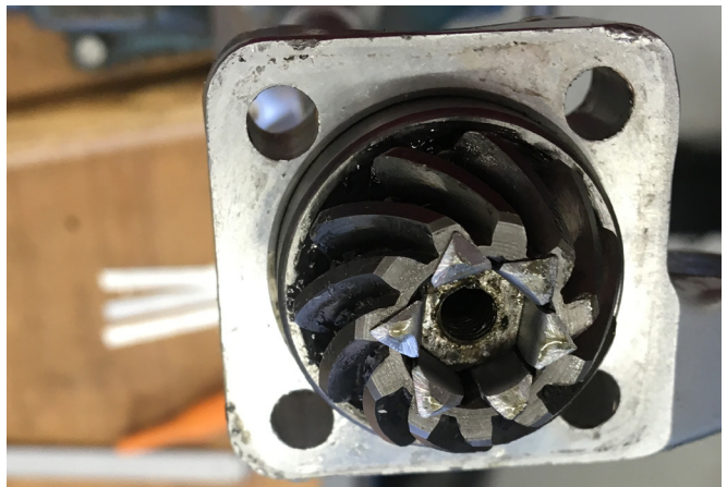
figure 216: The slack between the shaft drive and motor was removed by adding metal strips that fill up the gaps
