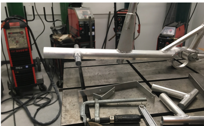
figure 193: The angles of the tubes were doublechecked after fastening the part with a spot weld. If the position was incorrect it could still be corrected using a plastic hammer. Only when the parts were in place they were welded together.
