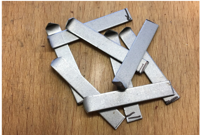
figure 215: Metal strips to fill up the gaps between the shaft and the sprocket
