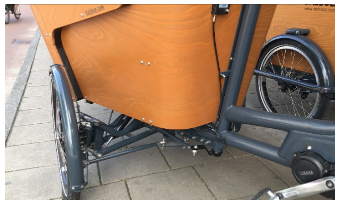
figure 157: The Babboe Carve also applies a caster angle
