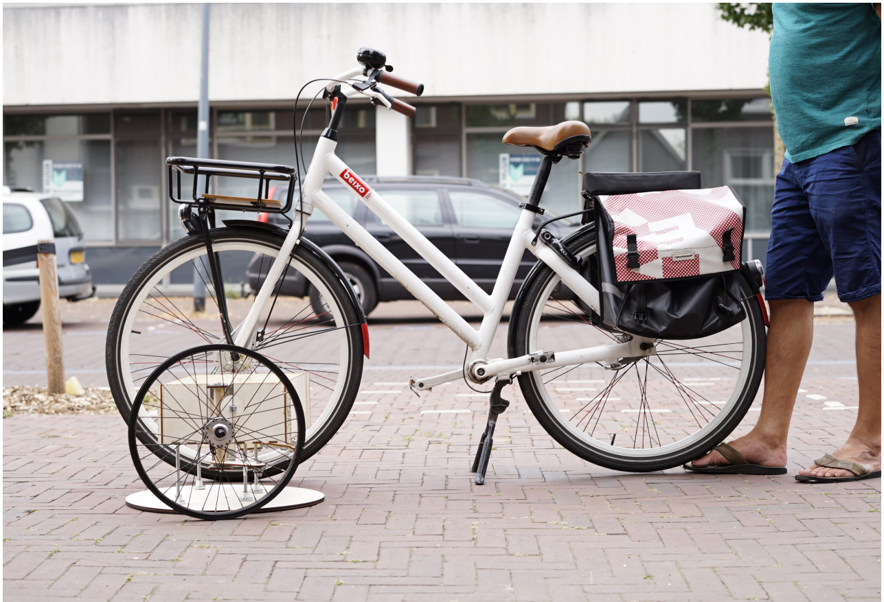
figure 68: 20 inch front wheels and 28 inch rear wheel
