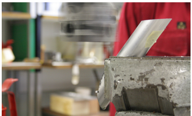
figure 188: The ends of the head tube, seat tube and reinforcement tubes had to be milled at specific angles to easily fit onto the adjacent tube to form the frame. This was done by using a boring head and placing the tube under the correct angle.
