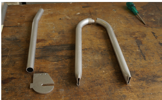
figure 187: The chainstay is made of a tube and a part used for connecting the rear wheel, mudguard and carrier. The seatstay consists of two bent tubes that are connected using a solid piece of aluminum which is welded in between.
