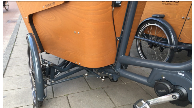
figure 123: Steering mechanism of Babboe Carve when on 'carve lock'
