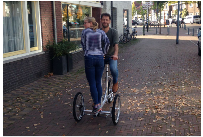
figure 211: The incorrect angle of the pivot arms led to positive camber
