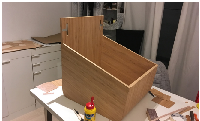
figure 209: In order to bend the veneer to be able to fit it on the base, it was made wet with warm water and clamped to the base. When it had taken on the shape, it was glued to the base and fixated with clamps.
