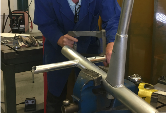
figure 214: To correct the position of the steering arms they had to be cut off
