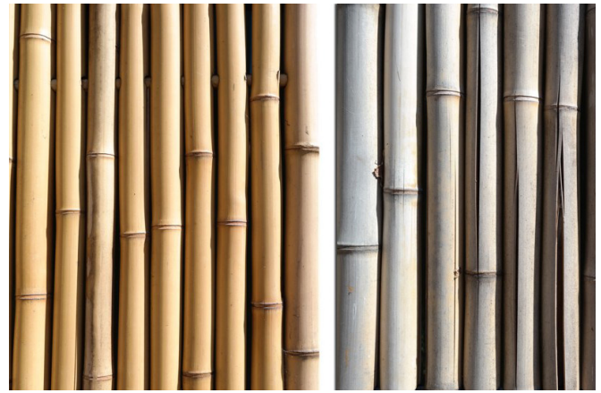
figure 150: Weather impact causes bamboo to turn grey (source: https://www.bambooiport.com/nl/blog/bamboe-eigenschappen-en-onderhoud )
