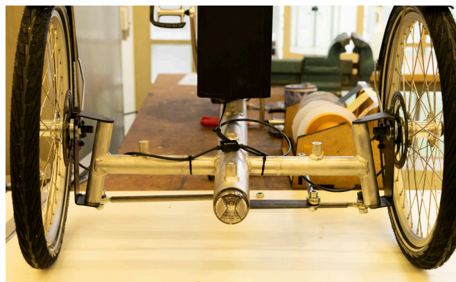
figure 200: The disk brakes were screwed to the attachment points on the pivot arm and the cables secured to the frame with tie wraps. Rubber sheet was attached to the side of the light to make it fit tight in the downtube. Attachment points for the container are welded to the frame.
