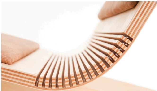
figure 169: Kerf bend applied to plywood (source: https://www.thebasicwood-working.com/how-to-bend-plywood/ )
