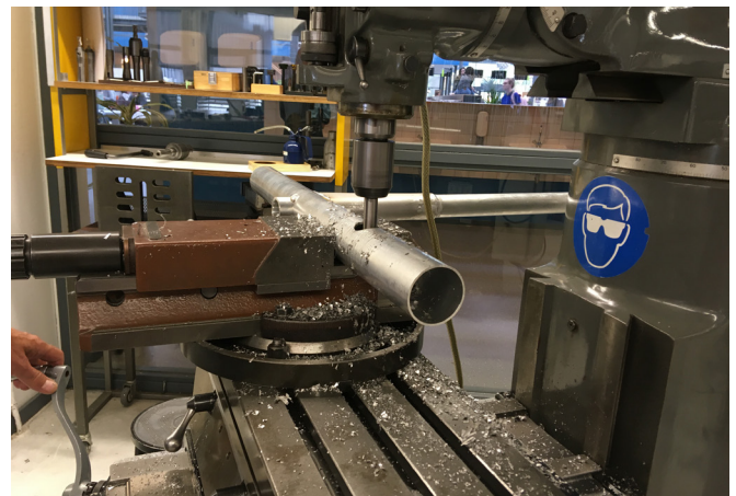
figure 213: To connect the steering arms a hole needed to be cut in the downtube
