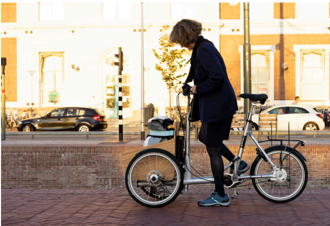
figure 164: The low entry and three wheels make getting on and off the bike easy
