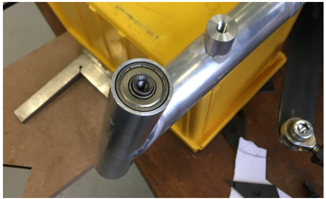
figure 195: The kingpin was created by pressing bearings in the top and bottom of the tube. A tube with internal thread was placed through both bearings and functions as axis. The pivot arms can be attached to the axis with two screws.
