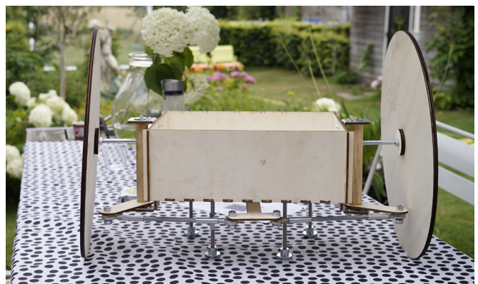
figure 128: The steering prototype does not fulfill all Ackermann criteria
