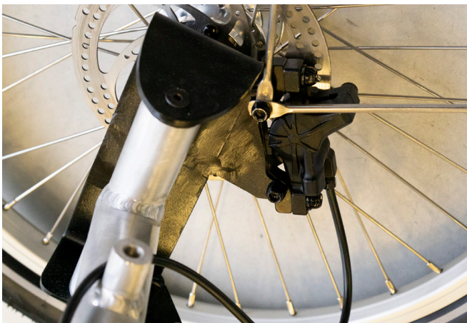
figure 212: The new pivot arm has a connection for the disk brake
