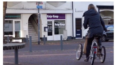
figure 234: The bike tilts in a turn without enough load
