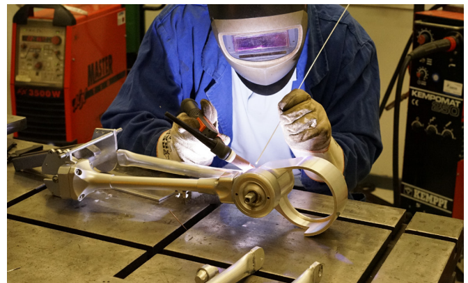
figure 192: The welding process started with welding the chainstay to the motorblock. Correct positioning was crucial.
