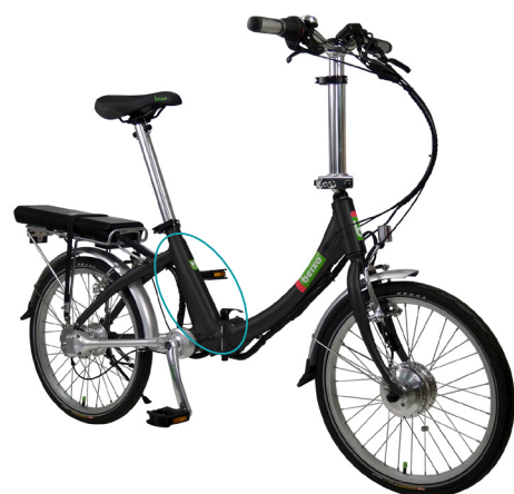
figure 106: Smooth transitions between the tubes make the frame stronger
