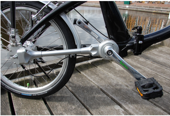
figure 4: Beixo bicycle with shaft drive (source: Beixo)
