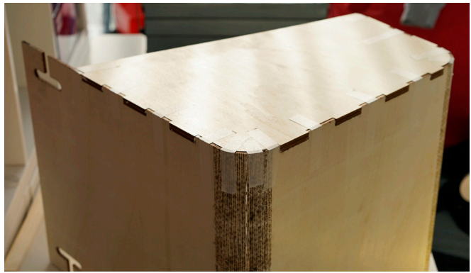
figure 168: Bending plywood using a lasercut pattern
