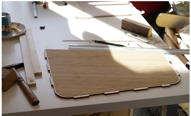
figure 207: After gluing the veneer on the side, the borders were cut off to allow for a good connection between the sides and the base.
