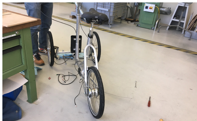
figure 204: The cables of the brakes, gears and motor were connected.
