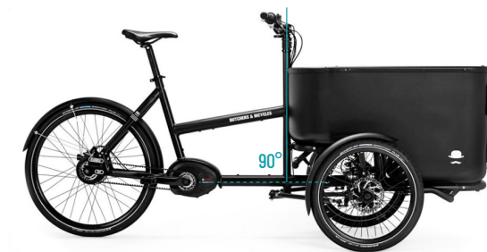
figure 73: This cargo bike has a head angle of 90 degrees
