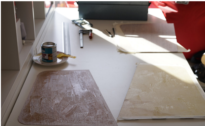
figure 206: The sides and base were traced on the bamboo veneer and cut with a stanley knife. The borders of the sides were covered with tape to avoid glue to stick. Wooden sticks were placed between the side part and the veneer to avoid that both will stick together at once. Then they were removed one by one.
