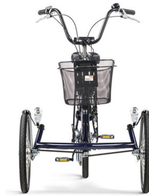
figure 158: The Huka trike applies kingpin axis inclination and neutral camber (source: https://www.huka.nl/en/products/ )
