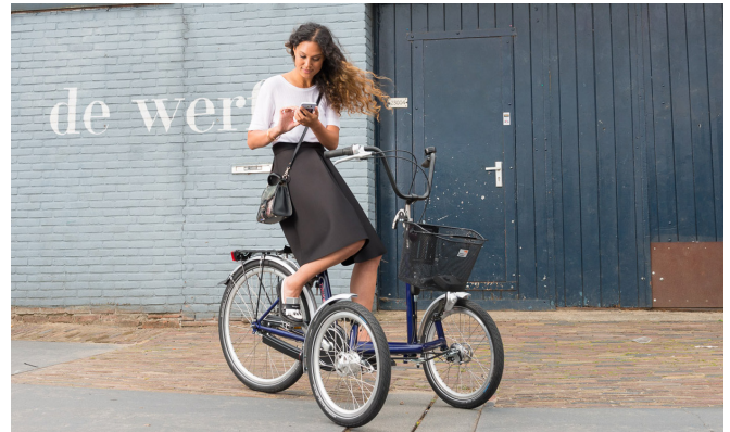
figure 155: The Huka trike applies caster (source: https://www.huka.nl/product/driewieler-trike/ )
