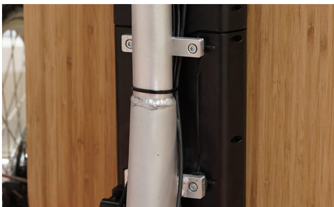
figure 201: Four connector points to attach the battery were welded to the headtube.
