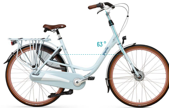
figure 72: The head angle of a city bike is smaller than that of a racing bike
