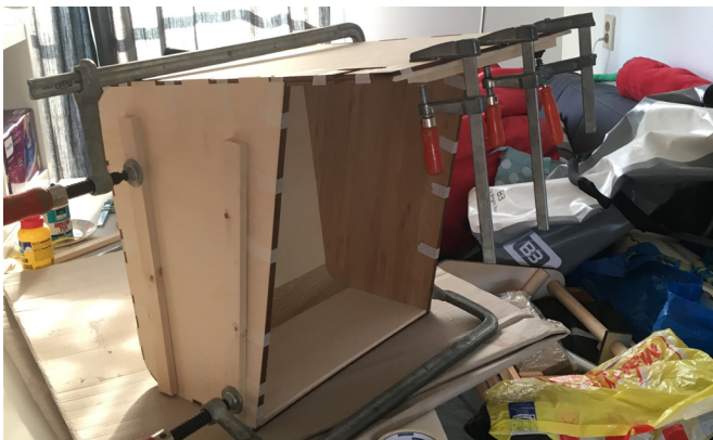
figure 208: Clamps were used to fixate the parts during the dryin process.
