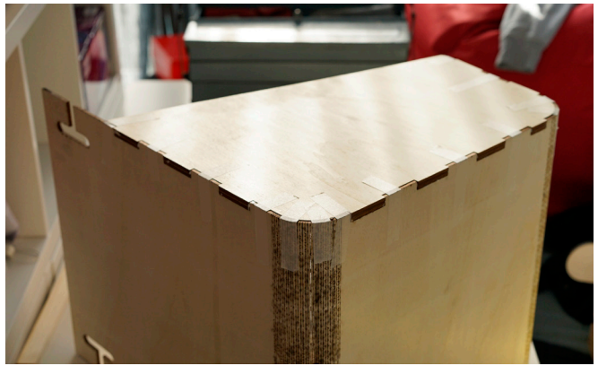
figure 205: A pattern of linear cuts made with the laser cutter was used to create a hinge and achieve the bent corners. A teeth connection also created with a laser cutter was used to attach the sides to the base.
