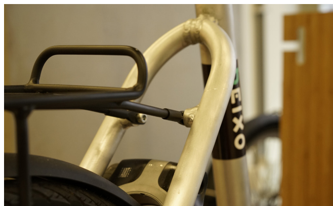
figure 202: Attachment points with internal thread for the carrier and the lock were welded to the seatstay.
