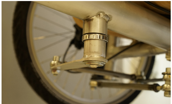
figure 197: The connection to the steering tube was created by welding a plate to a tube. It is kept in place with a screw and form enclosure and guided by a headset bearing.
