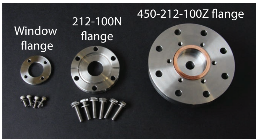
Figure A.14: Flange holding for the ZnSe input window.
